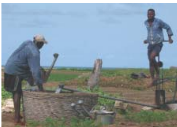
FIGURE 5: Water lifting via treadle and motor pump from tubewells into small tanks along the beach of Lome. A series of tanks can be connected through tubes to shorten distances for irrigation with watering cans (Photos: IWMI).
