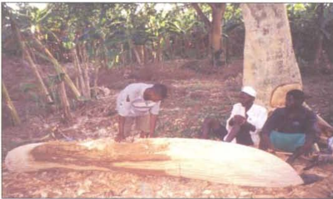
Making a canoe from the trunk of Ficus sycomorus , Mnazini, Tana River District
