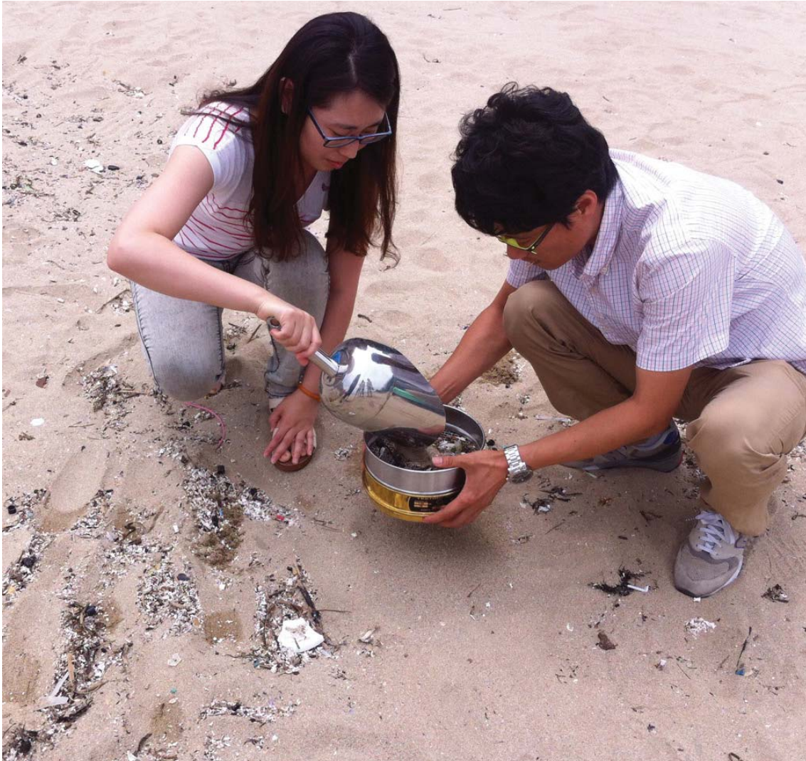
Sampling for microplastics on a sandy beach by dry sieving, near Busan, South Korea, July 2014. ©Peter Kershaw
