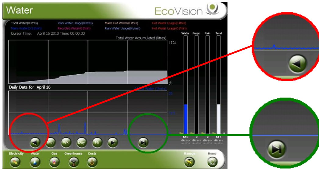
Fig. 6: EcoVision screen showing water usage page. Two sections are zoomed showing the water flow rates before (red) and after (green) a major water leak was fixed.
