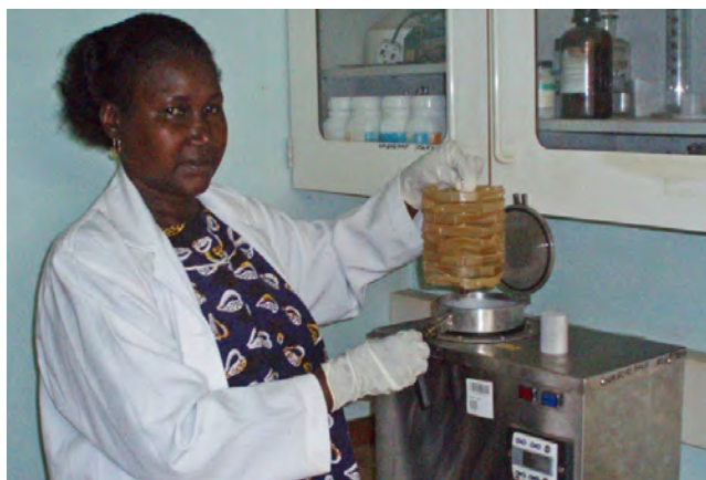
While a CRSP-supported MSc student at Sokoine University, Margareth Kibodya Mbwana helped with the laboratory analysis of Leucaena and Moringa leaf meals. In this particular test, she is determining their crude fiber content.
