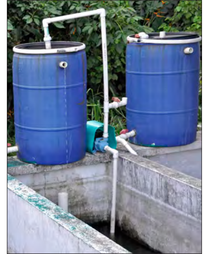
The CRSP MT-removal technology will scale-up from this simple filtration tank to commercial-sized systems capable of filtering MT-treatment water in large hatcheries.
