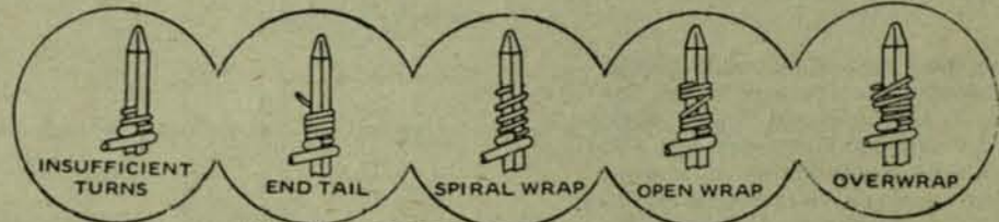
EXAMPLES OF INADEQUATE WRAPPED POSTS
