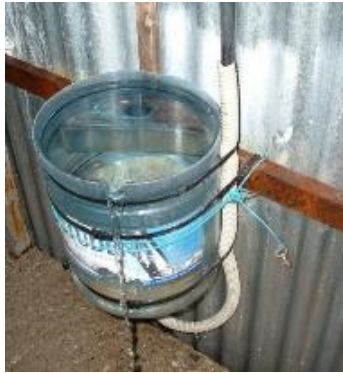
Hatchery jar made of "PET" bottle
