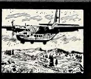
The Fairchild C-123 was especially designed for landings and take-offs on rough, unprepared fields.
