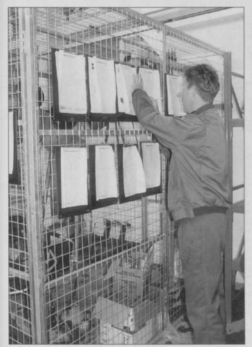
A check list is maintained for every machine. Note the security cage for storage
