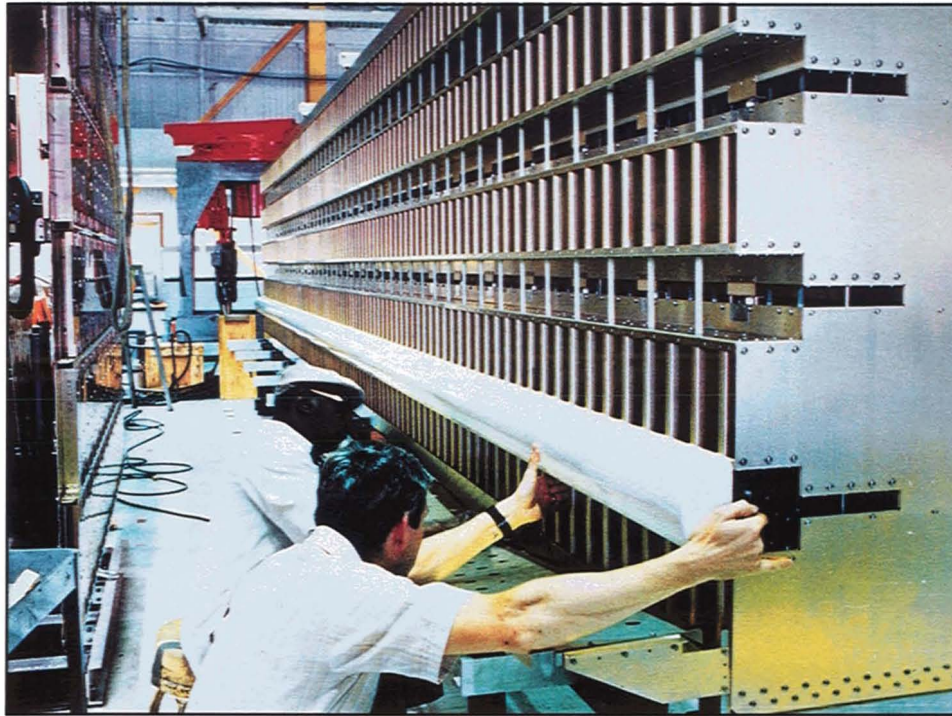
Fig. 6—Construction of the experimental four-row array. (Photo courtesy of Westinghouse Electric.)
