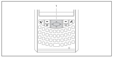
The way in which the navigation key (1) works depends on the application you are in. In some applications you scroll line-by-line up, down, left or right in a menu. To activate menu items press the middle of the navigation key. By contrast, in other applications – e.g. e-mail – you can page up or down with the navigation key.
