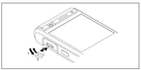
With the scroll button you can scroll up or down and forward or backward (1, 2) within the menu or application. You activate menu entries by pressing the scroll button in the centre position (3).
