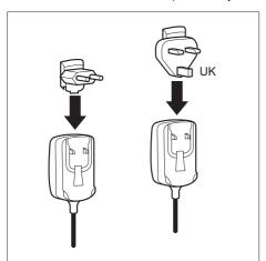
Slide the suitable mains adapter plug into the mains adapter in the direction of the arrow until it engages.
