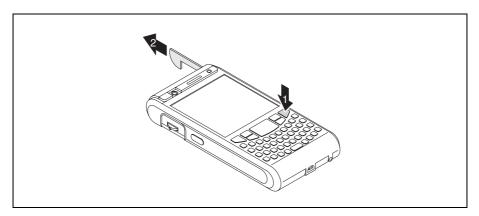
Press the End button to switch on the Pocket PC (1).
