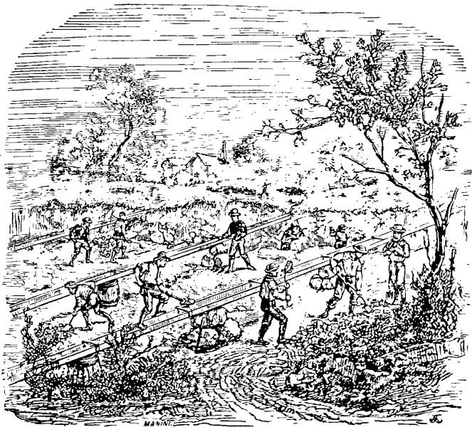
FIG. 2.—Simple Form of Placer Mining.
