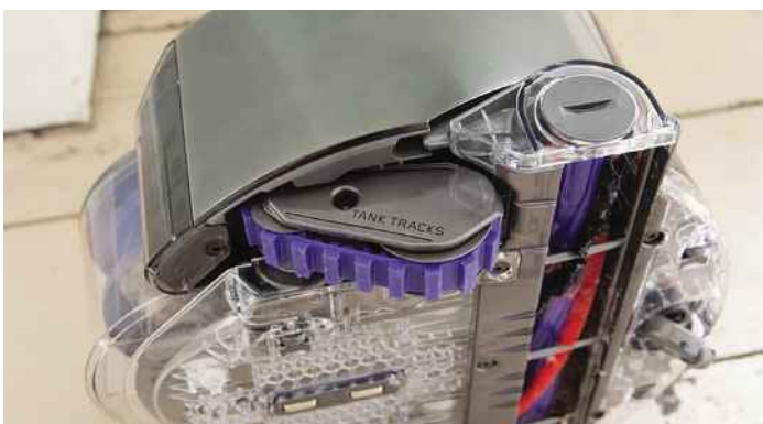
▲ Tank tracks at the back of the 360 Eye enable it to climb over any obstacles
