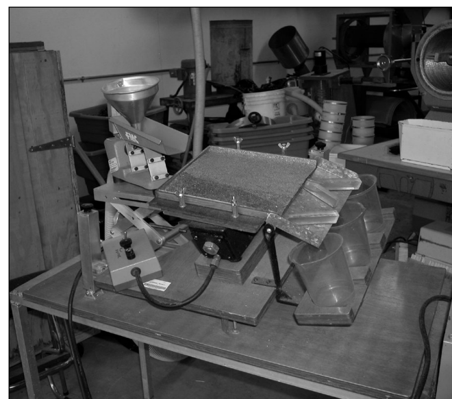
Figure 35 —Chapter 3, Seed Harvesting and Conditioning: the vibratory separator removes trash from seeds by differences in surface texture.
