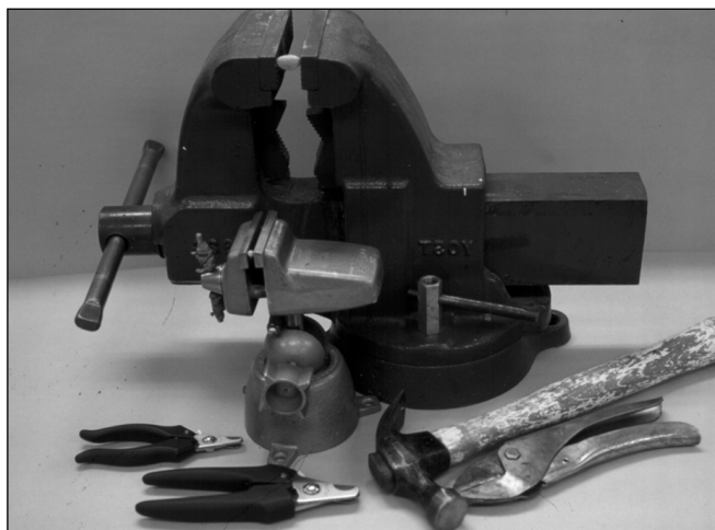
Figure 28 —Chapter 5, Seed Testing: vises, hammers, or clippers are used to cut through or remove hard or stony seedcoats for conducting tetrazolium or excised embryo tests.
