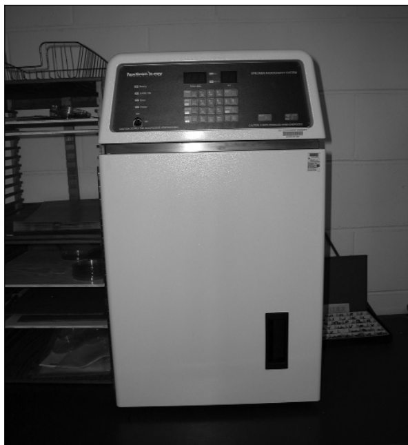
Figure 31 —Chapter 5, Seed Testing: a cabinet x-ray system is a safe and simple way to make radiographs of seeds.
