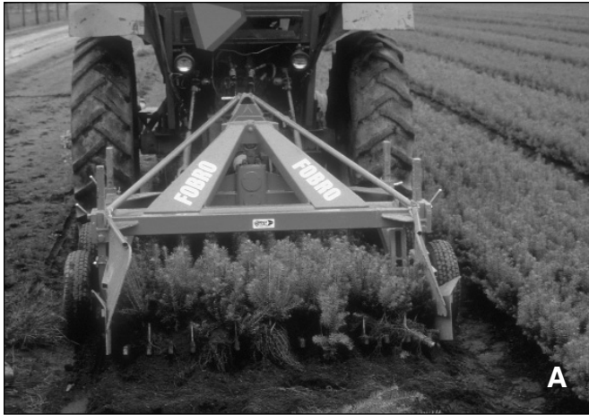
Figure 14 —Chapter 7, Nursery Practices: harvesting equipment lifts bareroot seedlings by undercutting them and loosening soil from around the roots with vibration ( A ). During hand-lifting, workers pull seedlings from the seedbed and place them in tubs, being careful to avoid excessive exposure and desiccation ( B ). Seedlings are then taken to the packing shed where they are counted and graded ( C ) to predetermined morphological specifications that were agreed upon by the nursery manager and the customer: shoot height, stem diameter (caliper), and some measure of root size and fibrosity ( D ). Finally, the “shippable” seedlings are sealed into moisture-retentive bags or boxes for refrigerated storage ( E ).
