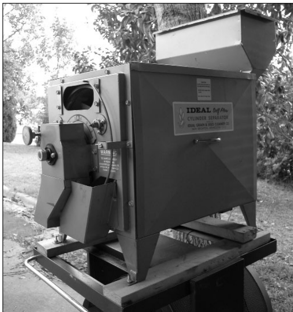
Figure 31 —Chapter 3, Seed Harvesting and Conditioning: indent cylinder machine for removing needles, sticks, and stems from seeds.
