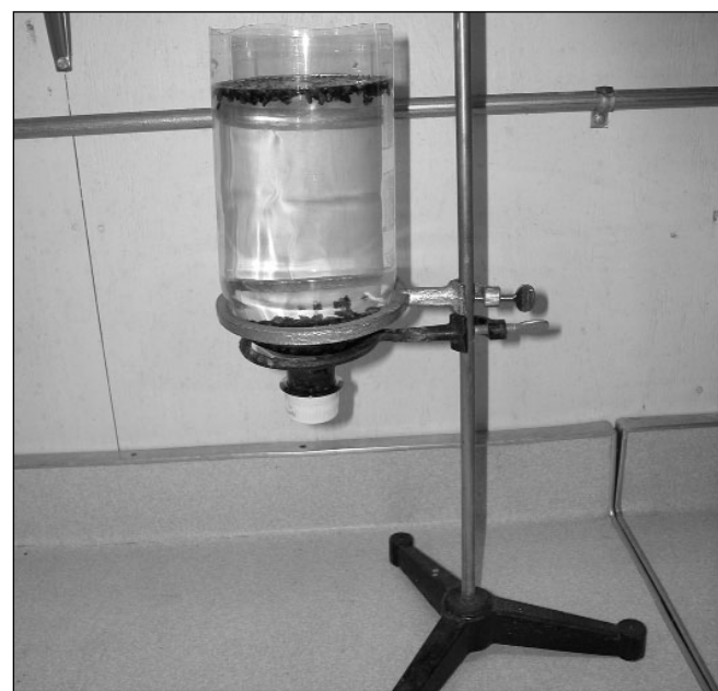
Figure 39 —Chapter 3, Seed Harvesting and Conditioning: incubate-dry-separate (IDS) separation chamber; the floating seeds are discarded because of low viability and vigor, and the sinking seeds are kept because they have higher viability and vigor.
