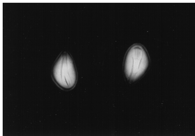
Figure 30 —Chapter 5, Seed Testing: x-radiography can be used to quickly determine how many seeds are empty, damaged, or poorly developed.
