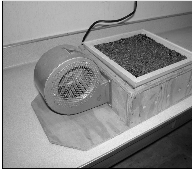
Figure 17 —Chapter 3, Seed Harvesting and Conditioning: laboratory model of a pressurized seed drier.
