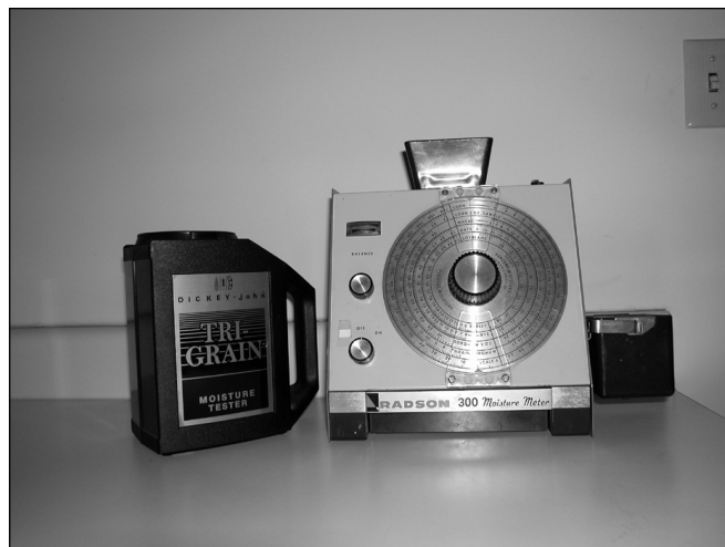
Figure 12 —Chapter 5, Seed Testing: electronic moisture testers can give a quick and reasonably accurate estimate of seed moisture.
