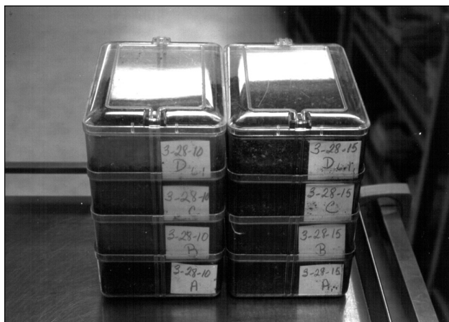
Figure 19 —Chapter 5, Seed Testing: 2 germination tests, each composed of 4 dishes containing 100 seeds each, the dishes are stacked for transport and prechilling.
