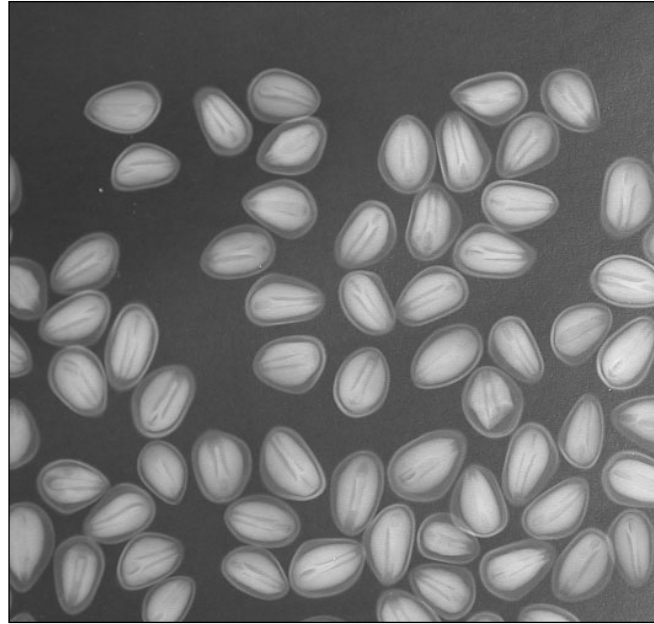
Figure 42 —Chapter 3, Seed Harvesting and Conditioning: radiography of pine seedlots quickly and accurately shows how many bad seeds to remove.
