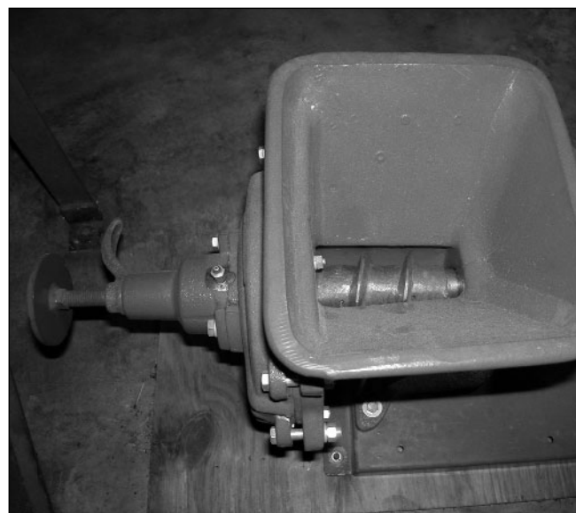
Figure 16 —Chapter 3, Seed Harvesting and Conditioning: a grinder can also be used to crush fleshy fruits for seed extraction.
