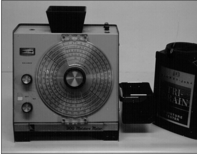
Figure 41 —Chapter 3, Seed Harvesting and Conditioning: electronic moisture testers are used to monitor seed moisture content.
