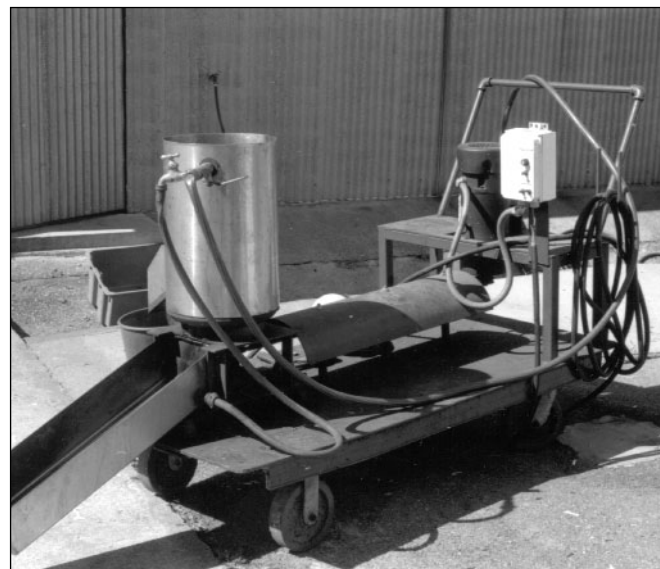
Figure 13 —Chapter 3, Seed Harvesting and Conditioning: a common type of macerator for de-pulping fleshy fruited seeds.
