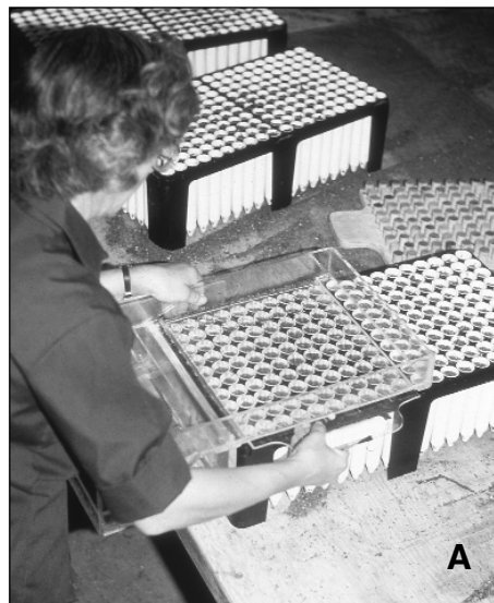
Figure 16 —Chapter 7, Nursery Practices: shutterbox seeders are custom-made for each type of container ( A ). Sowing consists of filling the precisely spaced holes in the shutter with seeds ( B, top ) and then moving it laterally to allow the seeds to drop into the containers ( B, bottom ).
