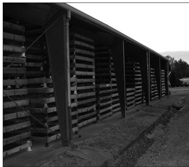
Figure 12 —Chapter 3, Seed Harvesting and Conditioning: screen bottom trays under shelter for air-drying dry fruits.
