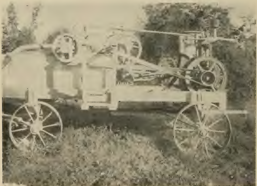
2. PRIMITIVE TYPE OF GASOLINE POWER SPRAYER, USED IN THE EARLY TWENTIETH CENTURY FOR CODLING MOTH CONTROL.
