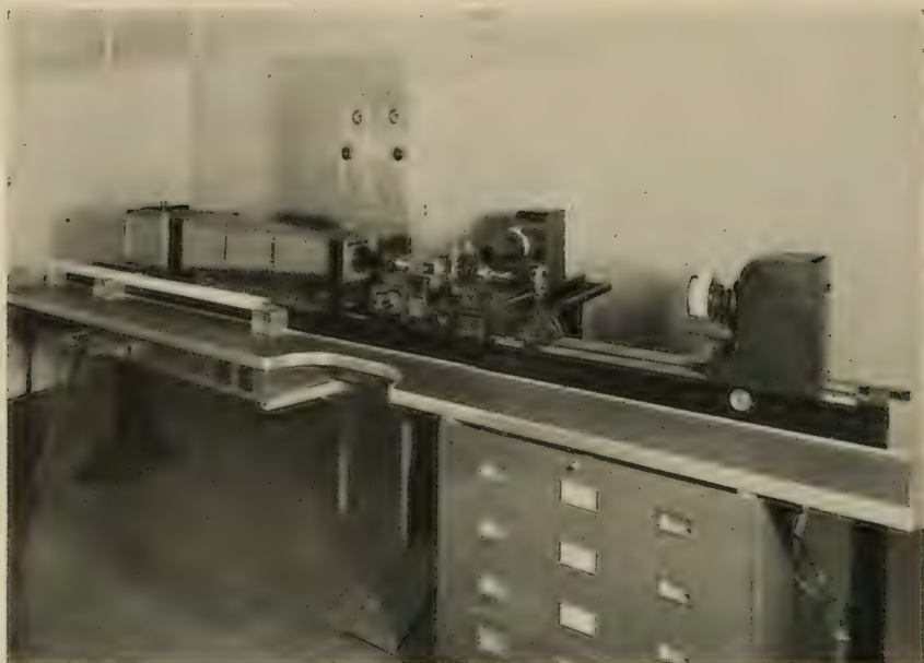
1. GENERAL VIEW OF GRATON-DANE PRECISION, ALL-PURPOSE MICROCAMERA.
