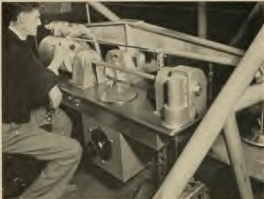
1. ENGINEER USING DYNAMOMETER FOR MEASURING MODEL RESISTANCE.
