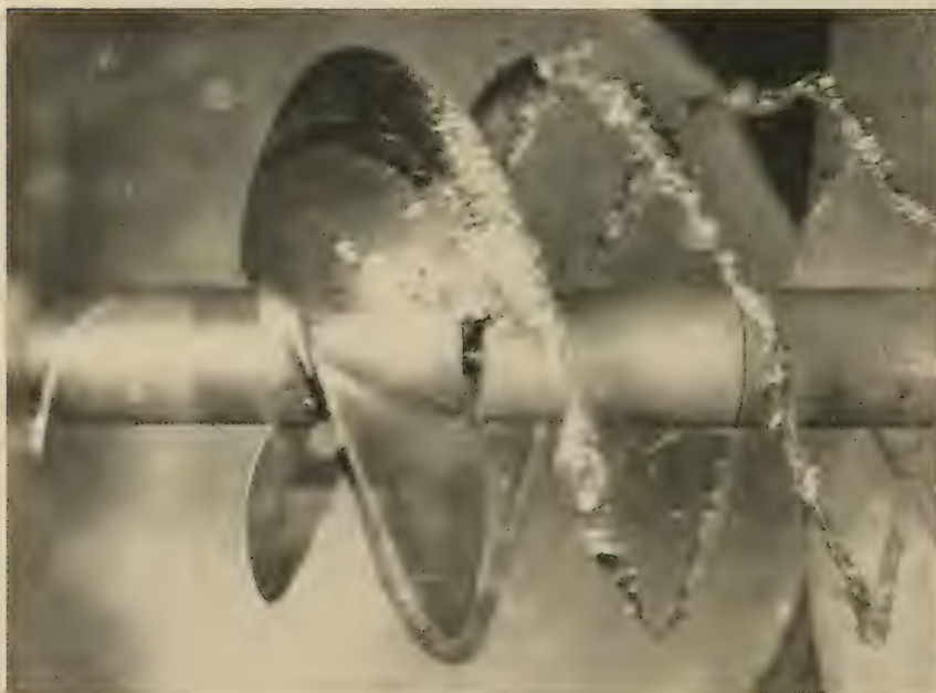
2. CAVITATING MODEL PROPELLER UNDER TEST IN 12-INCH WATER TUNNEL.
