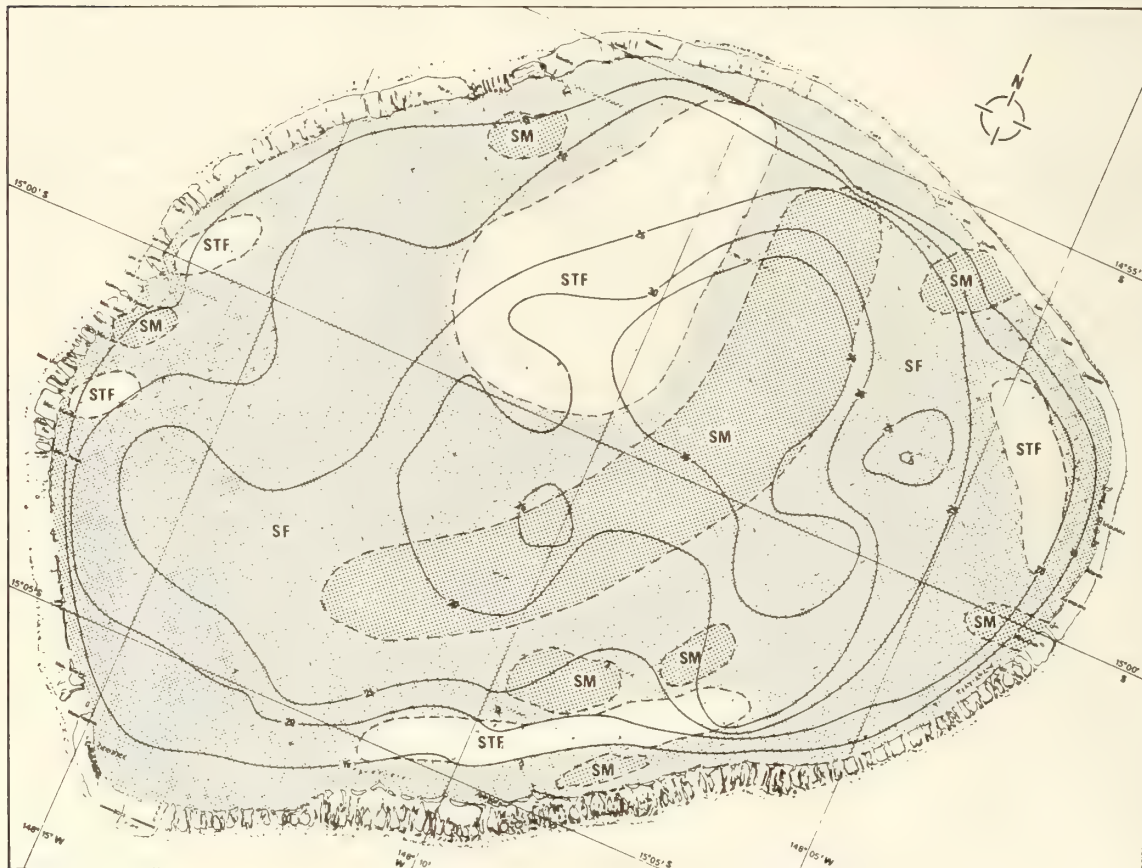
Fig. 10 : Contoured bottom sediment data of Tikehau lagoon characterized by mean sand size (STF : very fine sand, SF ; fine sand; SM medium sand; see text for definition of size-classes).
