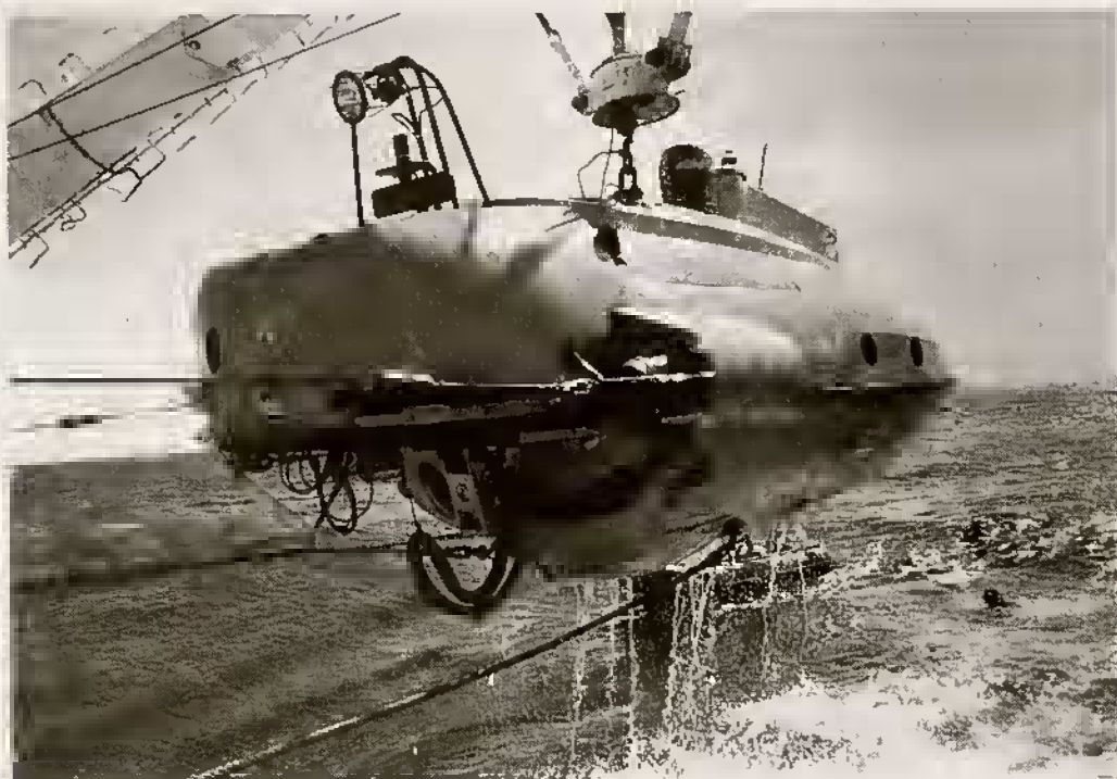
FIG. 1. — Recovery of SP 3000 Cyana at the end of a dive during the CALSUB cruise.
