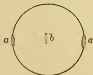
FIG. 1.—TWO ROUND COVER-GLASSES, cemented together with wax at a a , and having compressed between them an object b .
