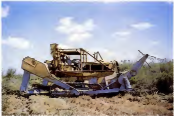
Plate 4. The King Ranch root plough. Note the scrub pusher in front and serrated blade on the rear root plough
