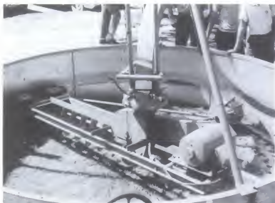
Figure 13.6. A top-unloading device for tower silos which excavates the silage and blows it into a trailer. Castor wheels centre and stabilize the excavator
