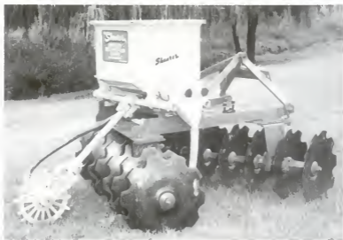
Figure 10.1. A grass seeder mounted on a tandem offset scalloped disc cultivator for seeding rangeland. The planting mechanism is operated by cable from the rear ground wheel
