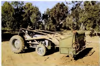
Plate 30. A home-made Cenchrus ciliaris (buffel grass) seed harvester. The height of the hydraulic end-loader frame on the tractor can be adjusted. The beater reel in the seed box has an 18-cm clearance from the floor; when the tractor is driven at 2.5 km/hour it beats off only ripe seed into the seed box. Seed is removed through the door on the bottom left of the seed box into bags
