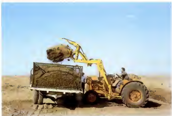
Plate 12. A grab attached to the end-loader of a tractor excavates silage from a trench and loads it into a truck for distribution
