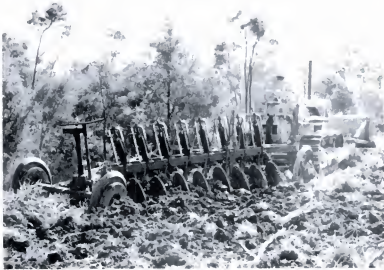
Figure 6.2. Heavy duty stump-jump disc plough removing Acacia harpophylla (bngalow) regrowth before overseeding the pasture
