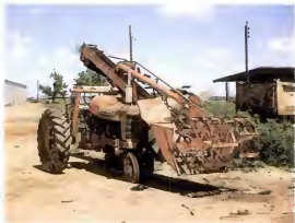
Plate 13. An excavator-elevator for removing silage from a trench and loading a following truck
