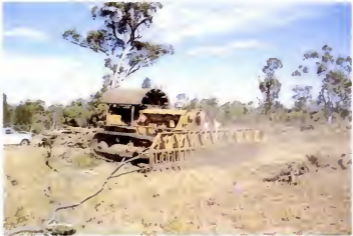
Plate 3. A scrub rake which pushes fallen timber into wind-rows. The spaced tines allow the soil to pass through
