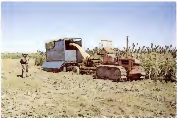
Plate 16. A crawler tractor pulling a forage harvester and side-tipping trailer harvesting sweet sorghum ( Sorghum bicolor cv. Saccaline) for silage. The full trailer is emptied by tipping it sideways hydraulically into a trench silo. At the end of each day the material is well compacted in the trench by the tractor
