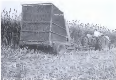
Figure 13.1. A combined chopper/catcher forage harvester for green chop
