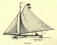
runners are placed at the ends of a runner-plank extend-ing across the frame at the point of its greatest beam, and the third is carried on a pivot at the atern and serves as a rudder.
