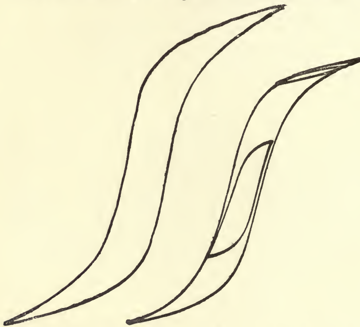
FIG. 56c.—Cyclic process of magnetisation automatically recorded by the Magnetic Curve Tracer.
