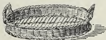
FIG. 159.—Wicker sieve for drying purified alum.
