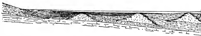
FIG. 86. Diagram showing successive advances of the coral reefs and accompanying clastic lime sands and the covering muds of the inner lagoons.
