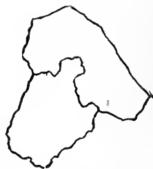
FIG. 171. Section across the two interlocking stylolites, shown in Fig. 172, much reduced. (After Wagner.)
