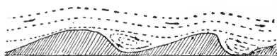
FIG. 141. Diagram showing direction of currents and vortices in the formation of ripple-marks. (After Darwin.)
