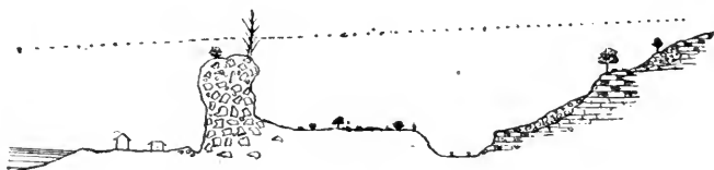
FIG. 117. Diagram illustrating the relation of the brecciated limestone to the bedded rocks at St. Ignace, Michigan. The stack is shown again in Fig. 118. The dotted line represents the hypothetical former extent of the brecciated material.
