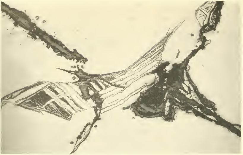
FIG. 1.—An irregular plessite field containing lamellae of taenite (gray) and small areas of incompletely transformed gamma-alpha aggregate. Small schreibersite bodies surrounded by hydroxide. Picral 85 seconds; \times about 35.
