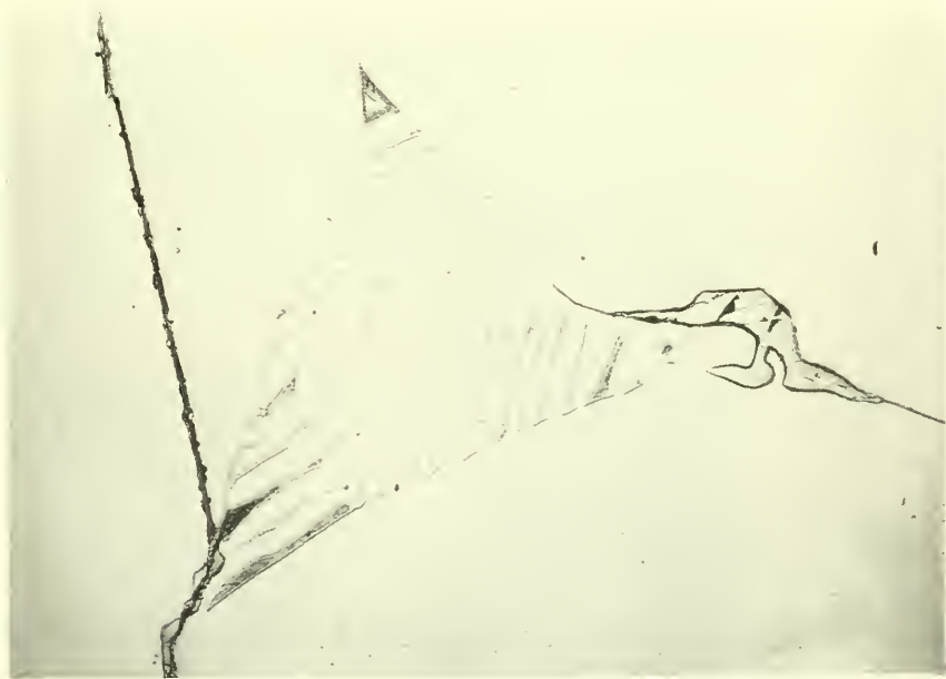
FIG. 2.—A light plessite field, the taenite lamella gray because of supersaturation with respect to kamacite. Picral 85 seconds; \times about 35.
