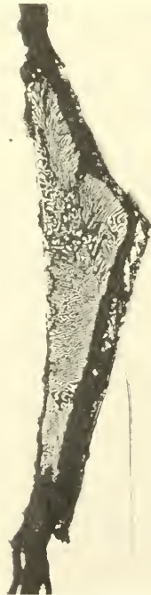
FIG. 2.—A plessite field with a pearlitic structure of kamacite and taenite lamellae, almost surrounded by hydroxide. At this magnification it resembles similar areas of pearlitic structure in a number of other irons (e. g., Leeds, Seelasgen, Youndegin) in which the white lamellae are kamacite and the gray are taenite. Picral 30 seconds; \times about 40.
