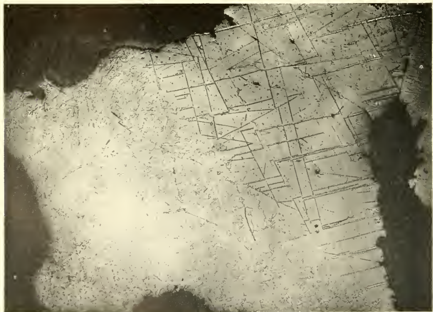
FIG. 2.—An area at the edge of the slice showing, at lower left, a zone of alteration in which the normal structure has been replaced by a secondary granulation. The dark area at lower right is probably hydroxide; that at upper left is silicate. Picral 120 seconds; \times about 30.
