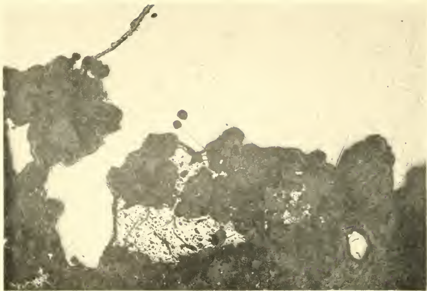
FIG. 1.—Irregular edge of an inclusion. The silicate at one point extends in a streamer from the mass. Three small isolated particles of silicate in kamacite. Picral 30 seconds; \times about 45.
