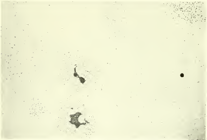
FIG. 2.—Sharply marked groups of phosphide particles, two inclosing dense areas composed of thickly crowded phosphide particles. Picral 40 seconds; \times about 35.
