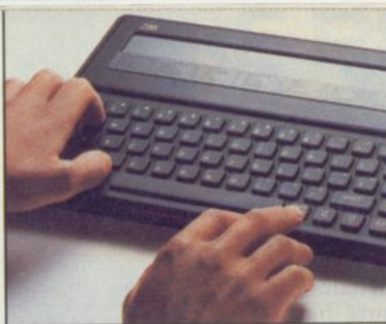
Full QWERTY keyboard offers 'silent', moving short-travel keys. Foldaway foot raises the Z88 12 1/2" for comfortable viewing and typing.
