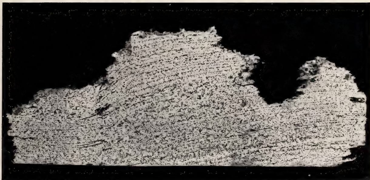
Figure 4: Douglas Fir panel, 30 cm long, exposed at Site 4 (70 m depth) for 4 months. Panel disintegrating due to massive wood destruction by Xylophaga washingtona
