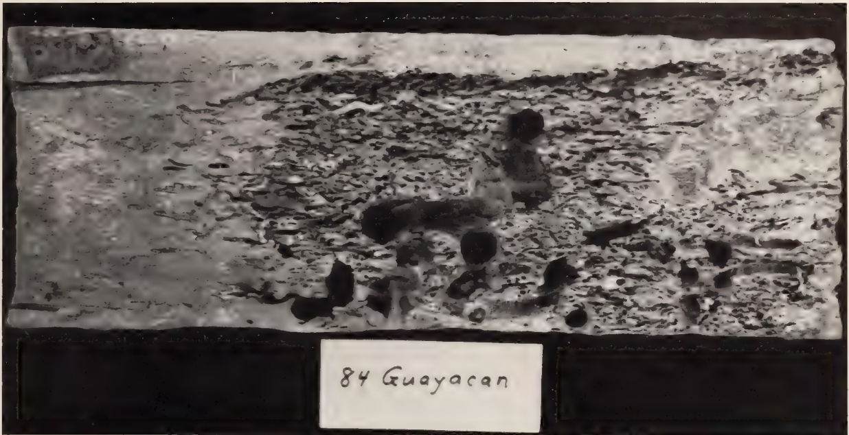
Figure 6: Guayacán panel damaged by Bankia setacea and Limnoria quadripunctata
