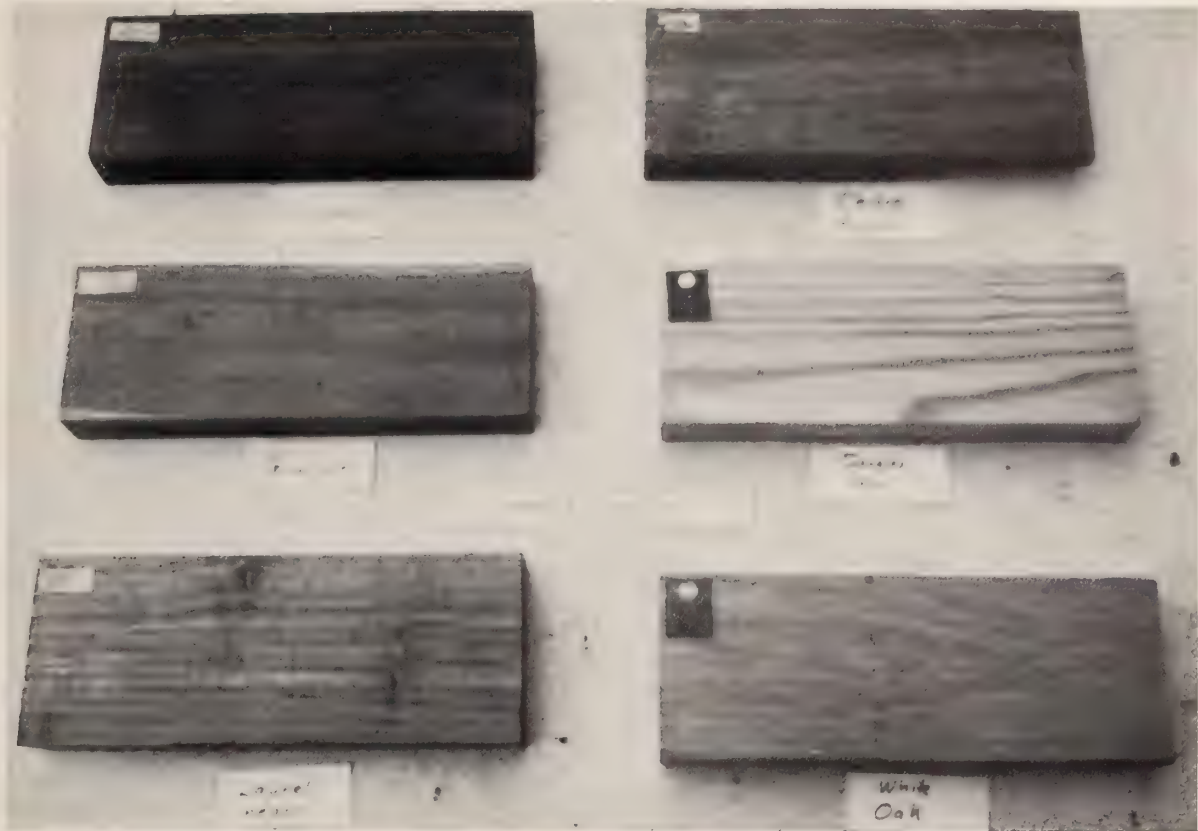
Figure 2: One set of wooden panels photographed prior to exposure in Monterey Harbor, September 1974. Each panel 23 cm long
