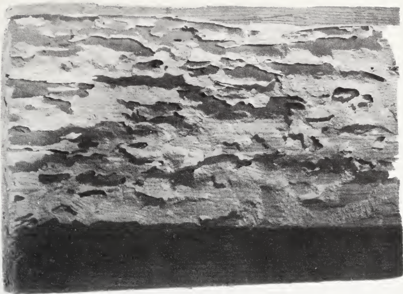
FIGURE 153.—Damage by the golden buprestid ( Buprestis aurulenta ) to a Douglas-fir timber.
