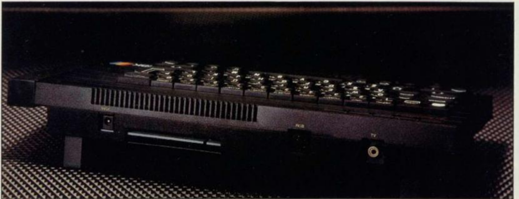
The RGB port on the rear of the machine will also provide a composite video signal.
