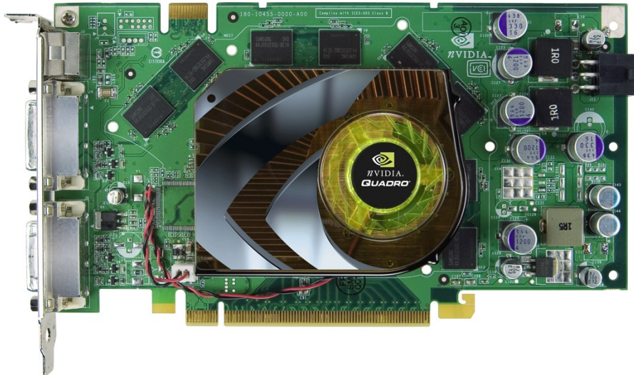
Figure 10– Board Layout of NVIDIA Quadro FX3700 Graphics Accelerator Card
