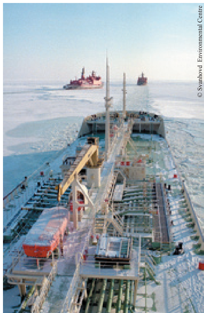
Figure 4.10 Small ice classed oil tankers operate the whole Northern Sea Route (in this report from Tiksi in the Eastern Siberia, the Laptev Sea to Murmansk in the Barents Sea). During winter these small tankers operate the ice covered ports of Varandey in the Pechora Sea and Talagi at Arkhangelsk and Vitino in the White Sea. This tanker is assisted by icebreakers.
