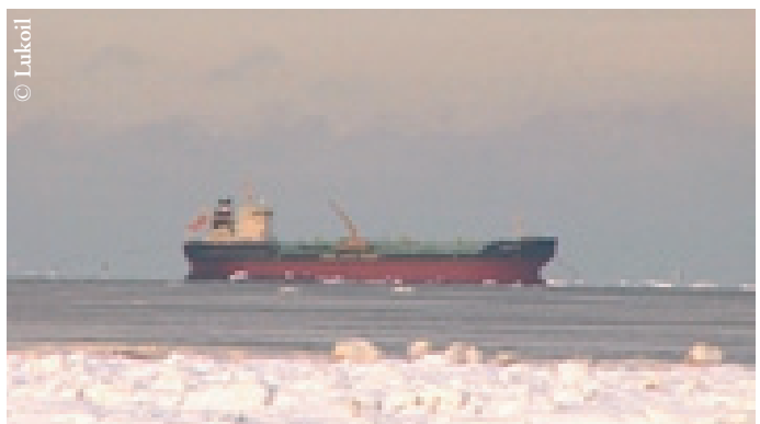
Figure 4.18 In 2004, two Lukoil Arctic Tankers Saratov and Usinsk operated on Varandey. These Astakhan -type tankers (20 000 dwt) have bow manifold and take oil from an underwater storage 4.8 kilometres off the coast. Lukoil plans to lay a 12 kilometre pipeline in the seabed to be able to load tankers up to 100 000 tons dwt.
