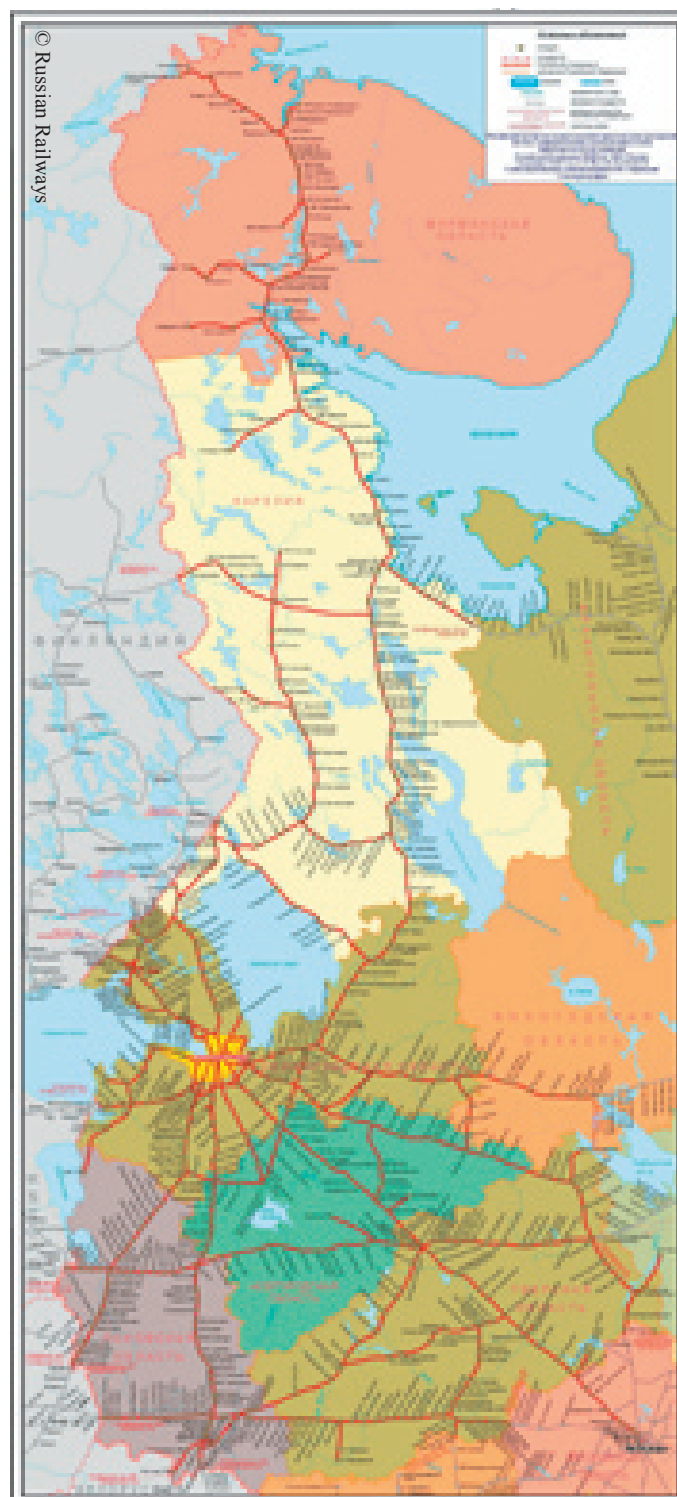
Figure 4.4 The October Railway operates from Moscow and Saint-Petersburg, north through Karelia to the city of Murmansk and westwards to the town of Nickel close to the Norwegian border. The railway line has an operational length of 10 143 kilometres and it carries more than 100 million of tons annually. The October Railway delivers oil products to Vitino and to Murmansk.
