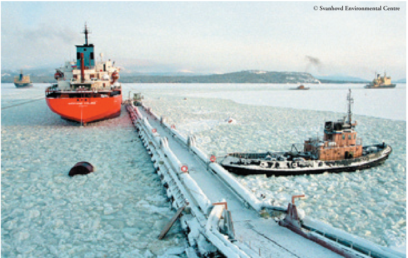
Figure 4.30 The Russian tanker Aleksandr Sledzyuk at the pier in Vitino during winter operation. The Lukoil Arctic Tanker Saratov is waiting to load. An icebreaker and two tugs are available for support.
