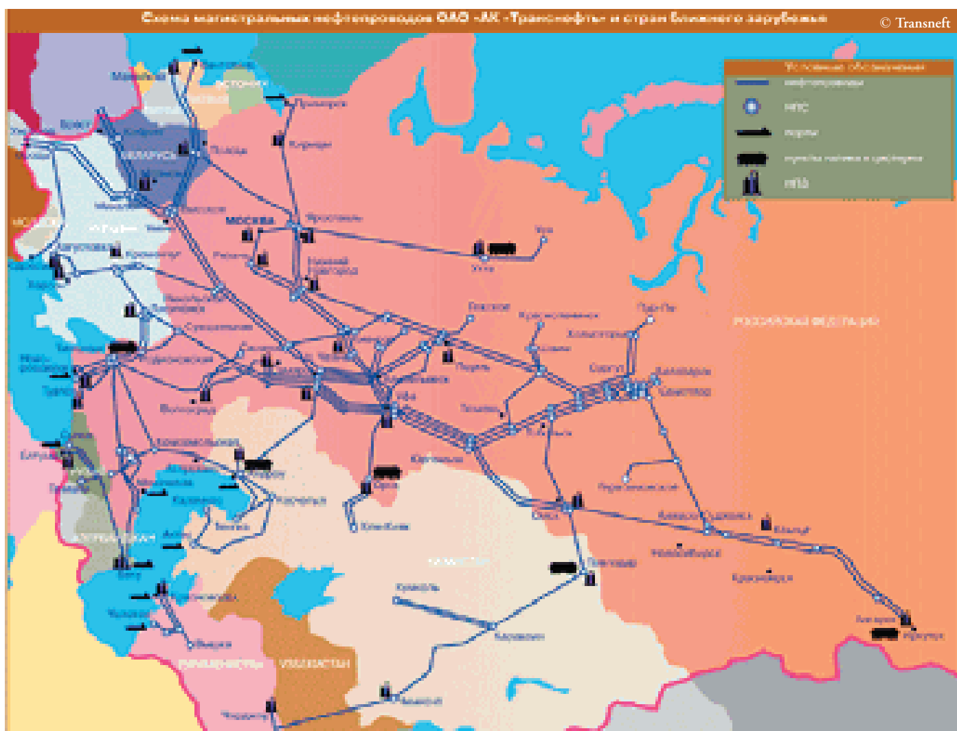
Figure 4.13 Transneft is the owner of the oil trunk pipeline system in Russia and may pipe 476 million tons of oil in 2005, sending 260 million tons for export.
