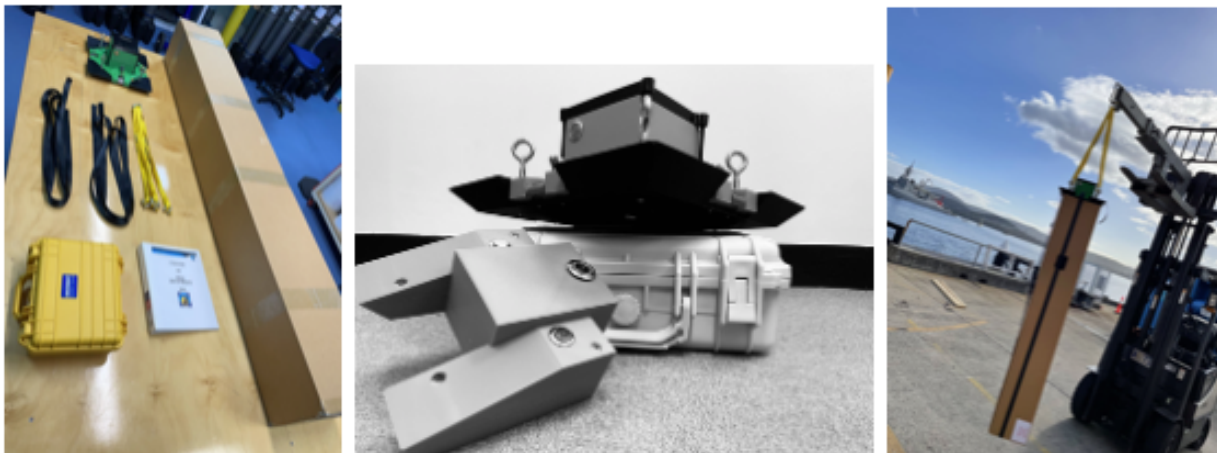
Figure 2: Photos of the Argo Release gear (left), the unit ready for deployment (middle), and a test on CSIRO’s wharf in Hobart (right).
