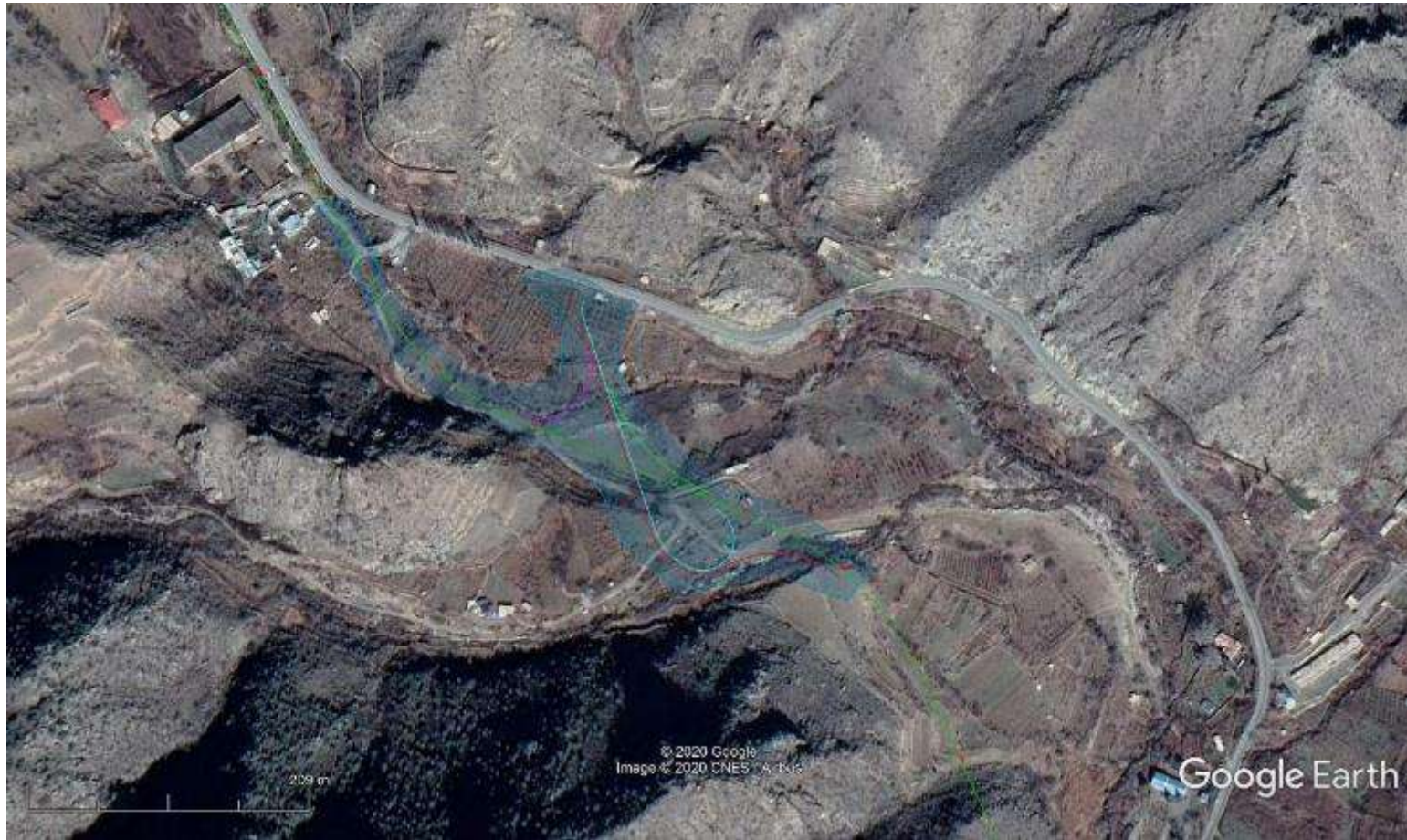
Figure 55: North-South highway route of the Meghri northern intersection and fords, on a photo taken with Google Earth. The boundaries of the direct impact of the highway on the natural environment (gardens, low river-bed ecosystem –G) are indicated in blue.
