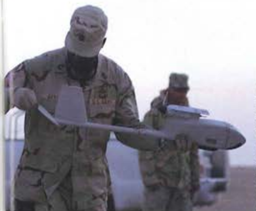
An intelligence analyst from the 3rd Infantry Division assembles the Raven unmanned aerial vehicle in preparation for a launch.
