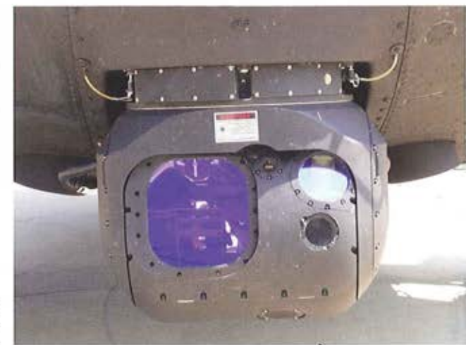
The Q2 is a lightweight, multi-spectral sensor with laser features, day and image intensified TV, here mounted under the cockpit area of a helicopter.
