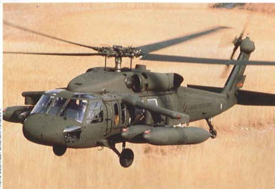
The UH-60 Black Hawk with the Crashworthy External Fuel System (CEFS)
