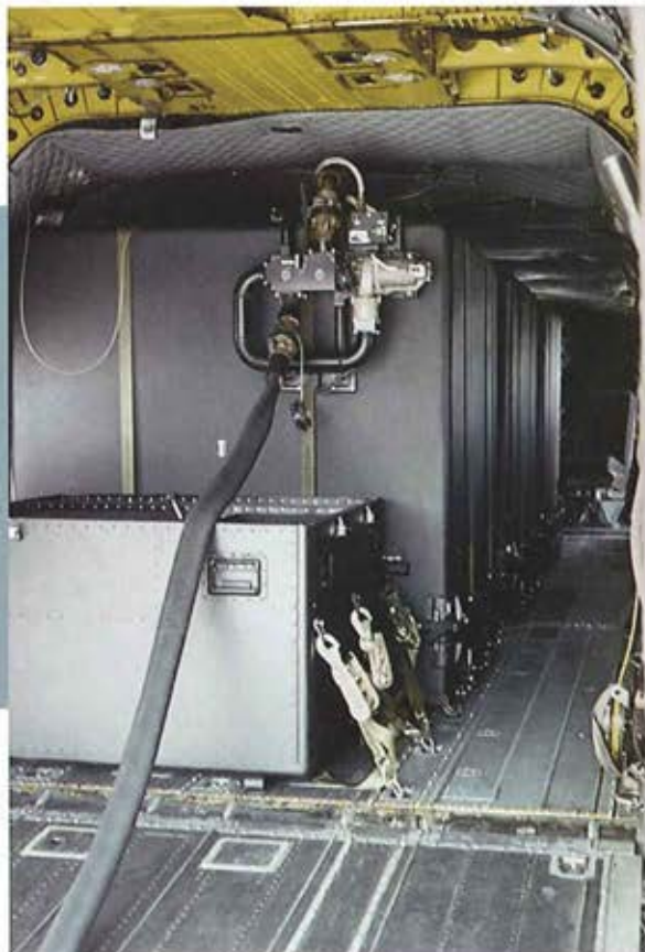
The CH-47 Chinook Extended Range Fuel System II (ERFS II) can be used for internal refuel or external fueling operations for other aircraft or weapon systems.
