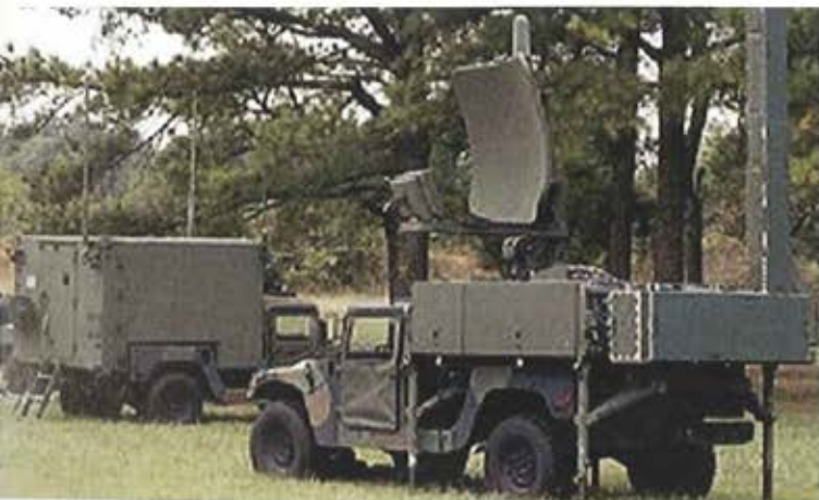
The Air Traffic Navigation, Integration and Coordination System or ATNAVICs is a highly mobile system providing air traffic services to remote locations where no operational airport control and landing system exists.
