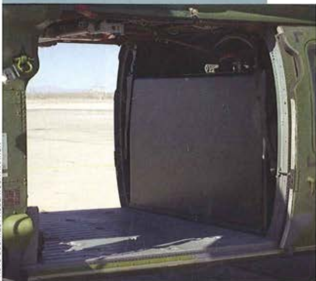
The GUARDIAN® 200 single Internal Auxiliary Fuel Tank System installed against the aft cargo area bulkhead of a UH-60 helicopter.
