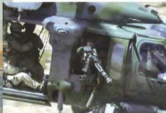
A US Air Force HH-60 helicopter equipped with the M134 mini-gun. This system would allow the UH-60L to perform self-escort on routine general support missions which currently, because of threat, require armed escort.
