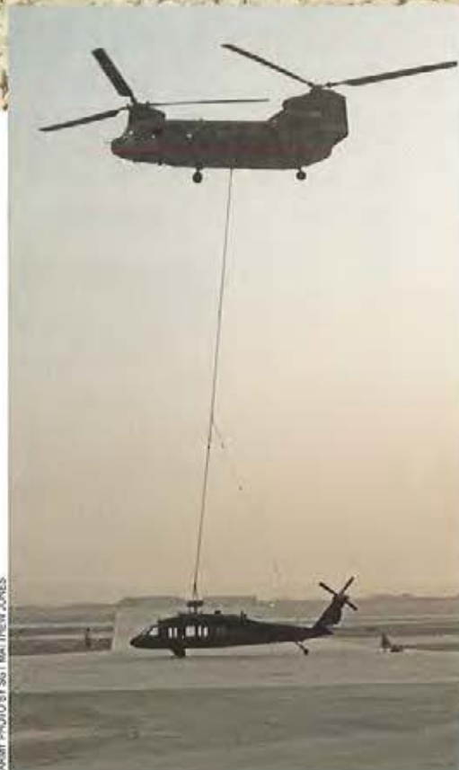
A CH-47 Chinook conducts a sling-load operation along the flight line on Contingency Operating Base Adder.
