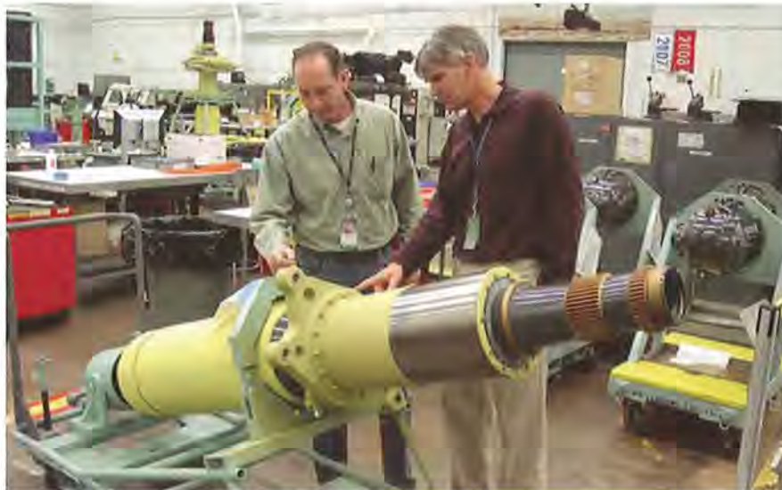
CW3 Jerry Irick (left) and Joe Huppman (lead QA Inspector) in Boeing's Dynamics Center discussing the finer points of a CH-47 aft vertical shaft. The Dynamics Center assembles, paints and tests transmission components and rotor heads for the Chinook.
