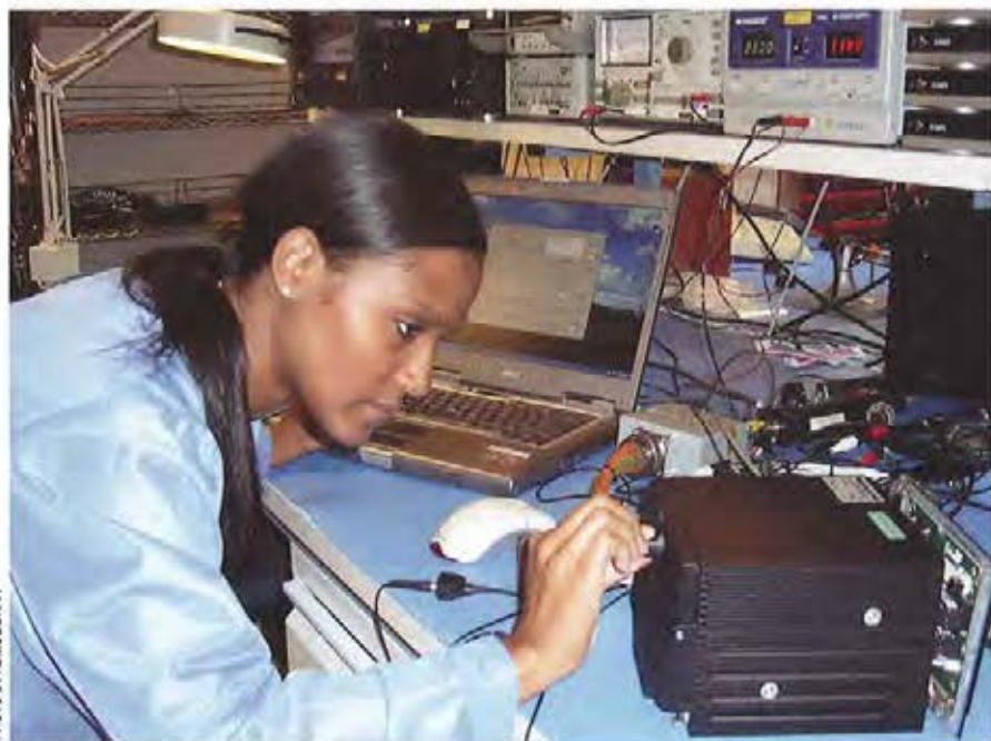
A technician at Goodrich's Sensors and Integrated Systems business in Monterrey Park, California performs acceptance test procedure on a mission data recorder.
