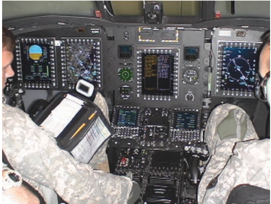
Students at the U. S. Army Aviation Center of Excellence train in the CH-47F Transportable Flight Proficiency Simulator.
