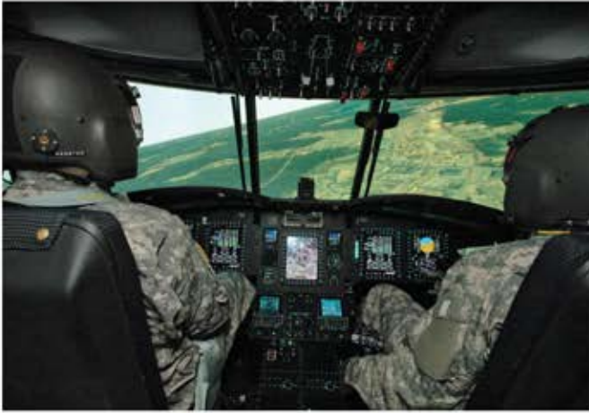
CH-47F Flight School XXI simulator during an in-factory systems performance assessment.
