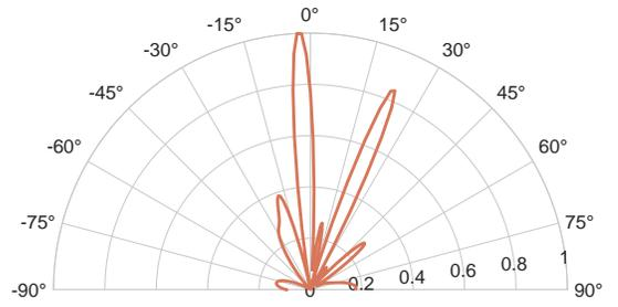
Fig. 4. Radiation pattern of the one-dimensional RHS.
