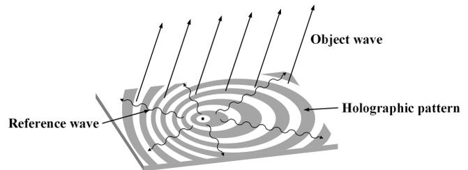
Fig. 1. Illustration of the holographic antenna [3].
