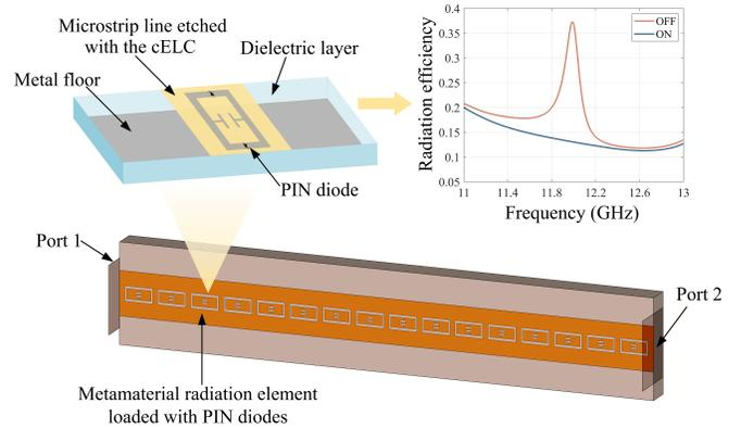
Fig. 3. Illustration of the metamaterial radiation element and the RHS simulated in the CST software.
