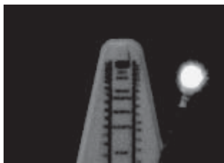
Fig. 9 Photograph of an operating metronome, which was taken by the trial product of the proposed organic CMOS sensor without micro color filters.
