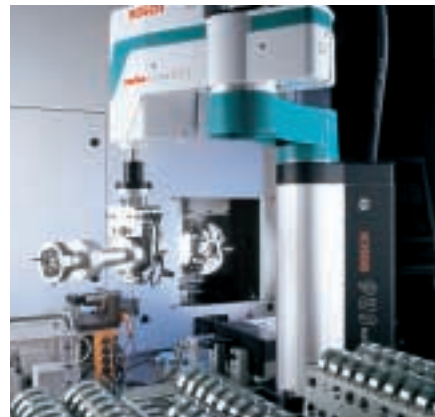
We developed and in 1998 introduced a completely new generation of our proven robot series Turbo-scara. These swivel-arm robots are particularly robust and efficient.
