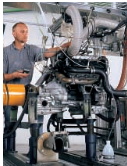
Taking measurements of a diesel engine in the Stuttgart-Feuerbach plant. In this test room injection components are tested under actual engine operating conditions.
