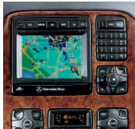
We developed the electronic driver information system Comand (Cockpit Management and Data System). It includes a dynamic navigation system which changes the selected route to take traffic conditions into account, and also incorporates a number of operator functions.
