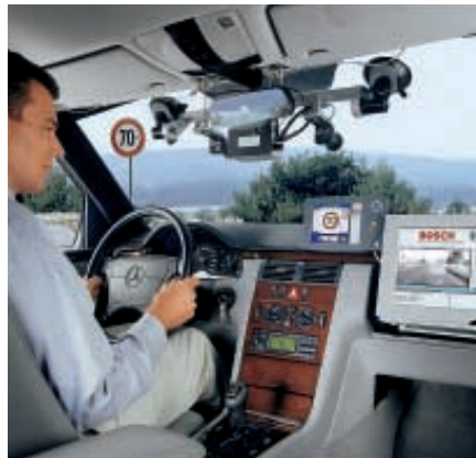
Bosch is intensively working on videosensorics for motor vehicles. One important use is the Traffic Signal Assistant, which by means of visual or audible signals draws attention to traffic regulations, such as speed limits.
