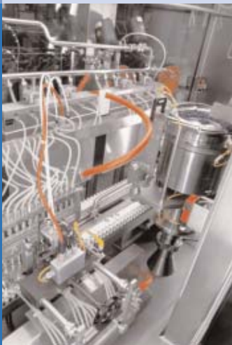
Highly demanding insulator technology for the pharmaceutical industry from Bosch: equipment for cleaning, sterilizing, filling and closing of ampules.
