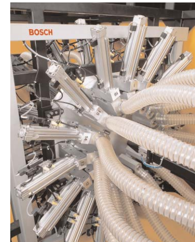
Bosch pneumatics for plastics processing: units consisting of pneumatic cylinder, solenoid valve and cylinder mount guarantee fully automatic material flow.
