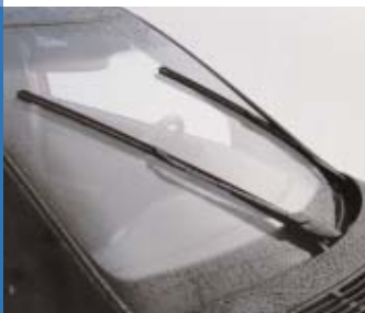
Innovation for the windshield wiper. Our new hingeless wiper blade presses the wiper rubber against the windshield by means of two tension strips. The uniform distribution of pressure improves wiping quality, especially at high driving speeds.
