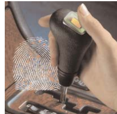
Drivers can be unequivocally identified by means of biometric processes such as fingerprint detection based on physiological features. A fingerprint detector integrated in the gear selection lever replaces the ignition key. As soon as the driver's thumb print identifies him as an authorized user, the sensor's surround lights up and the engine can be started.
