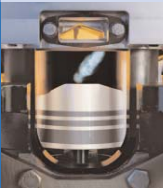
Mixture formation in the gasoline direct-injection engine takes place in the combustion chamber. We analyze the process with laser spectroscopy in an engine.
