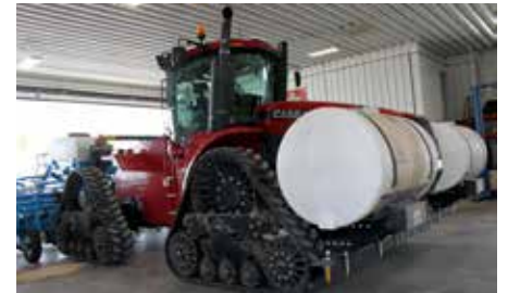
A Rowtrac version of the Steiger Quadtrac 400 helps minimise soil trafficking and crop damage in rowcrops.
