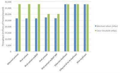
Figure 2: Comparing Cisco Cloudscale and merchant silicon throughput
