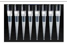
All liquid levels are similar in volume and opacity without air trapped in the pipette tips.
