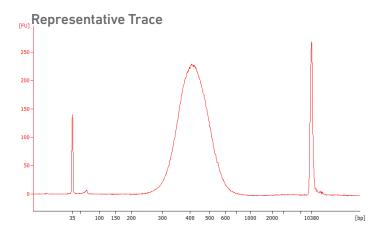
Determine the average fragment size from the Bioanalyzer trace. This will be used as the insert size for library quantification.
