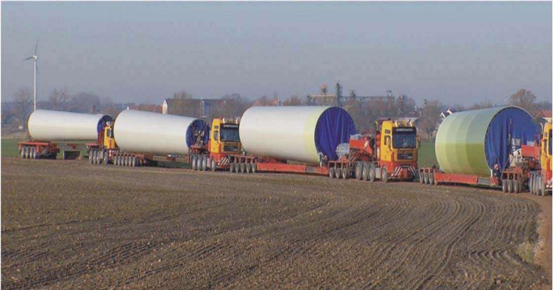
Figure 13.1: Typical Delivery of Wind Turbine Tower Components
