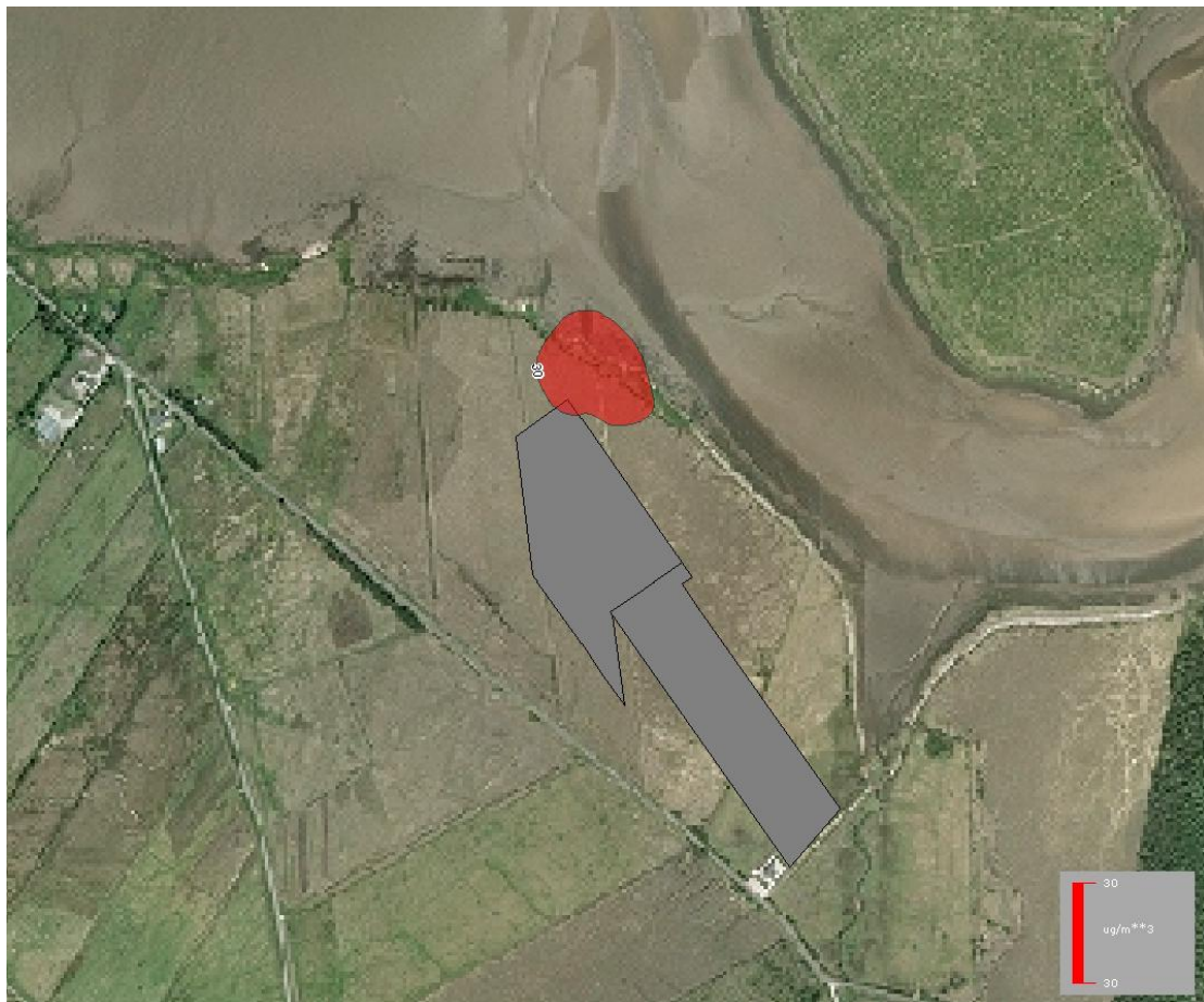
Figure 2: Annual Average NO x emissions from the generators on the tunnel compound – Worst Case Scenario where generators are at nearest boundary to cSAC.
