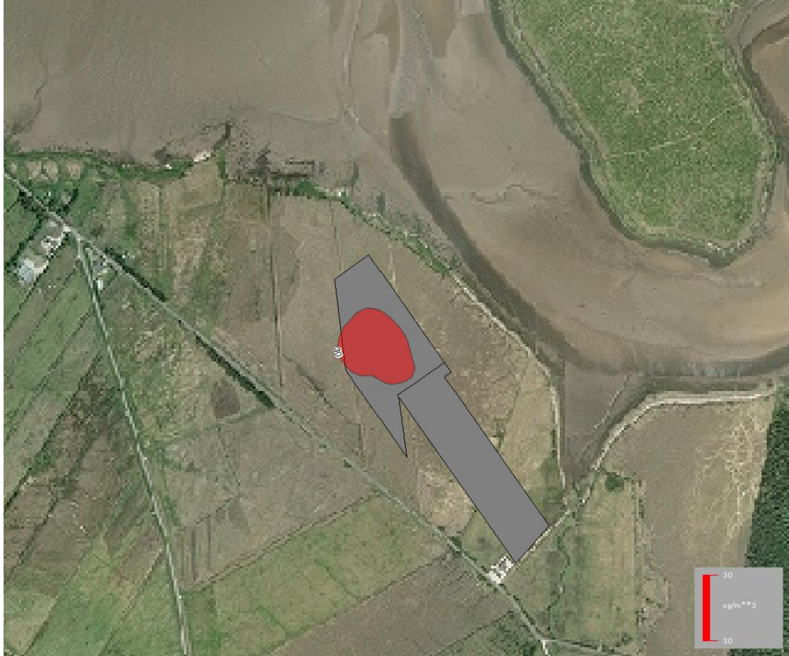
Figure 3: Annual average NO x emissions from the generators on the tunnel compound – Most Likely Scenario where generators are located as per Figure 5.7.
