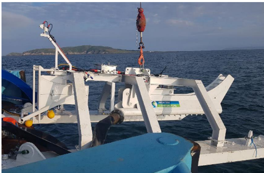
Figure 17 (a) Sandpiper sled mounted jet trencher
