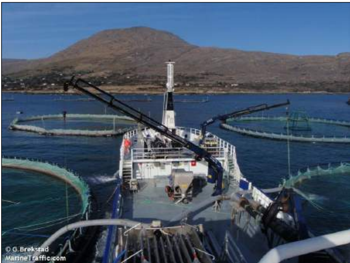
Figure 2-19: The proposed well boat MV Grip Transporter distributing fish to two pens (© Magnar Lyngstad, MarineTraffic.com).
