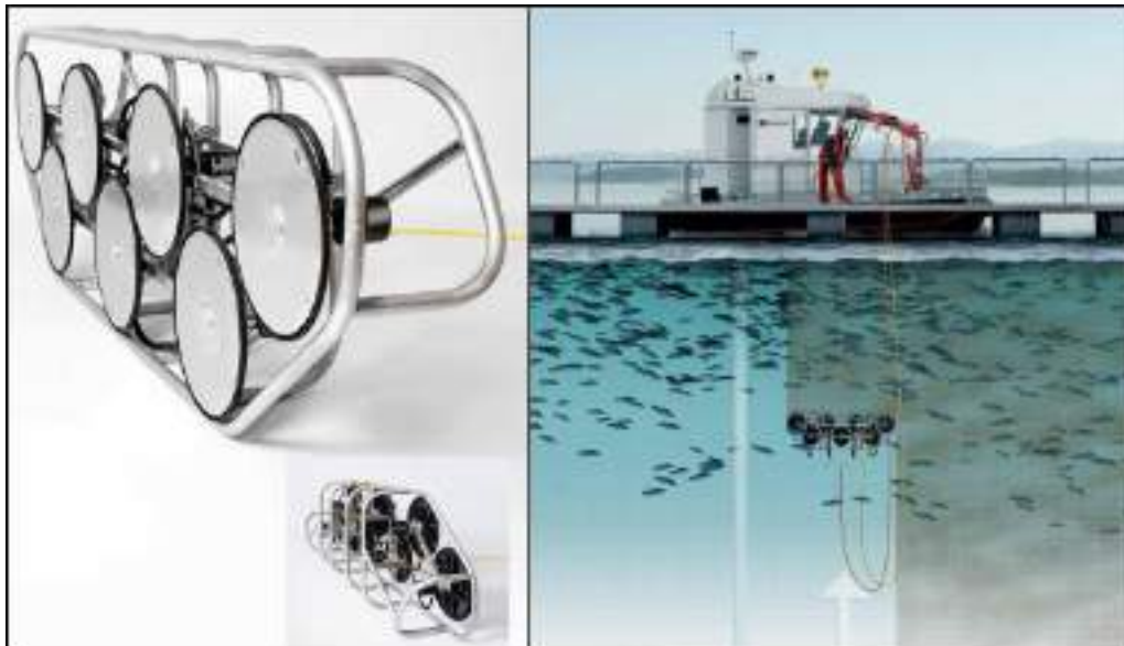
Figure 2-10: Net cleaning with the IDEMA net washer (© Akvagroup; www.akvagroup.com ).
