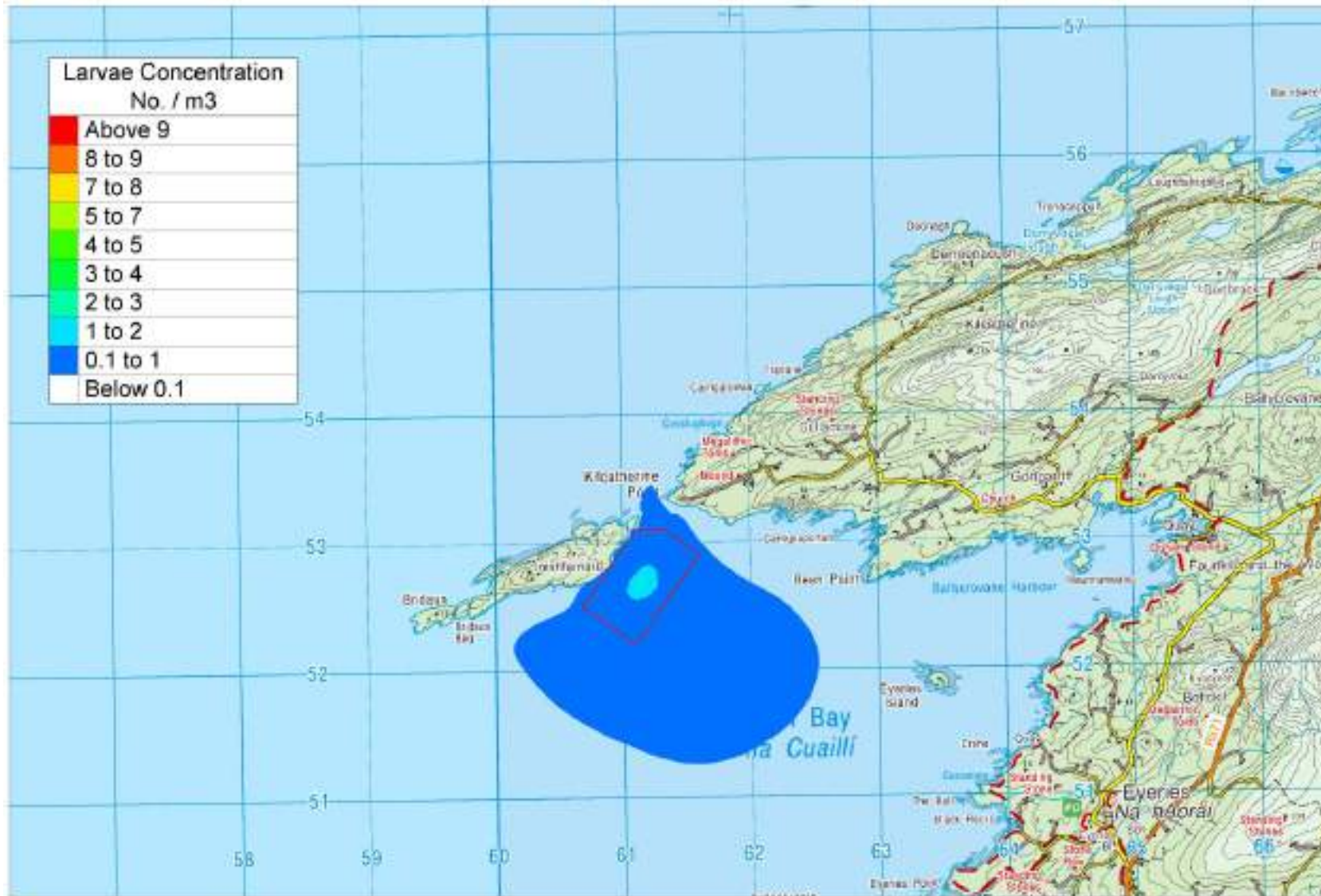
Figure 6-13: Predicted tidal mean Nauplius I larvae numbers (No./m3) from the Inishfarnard Farm Production Site.
