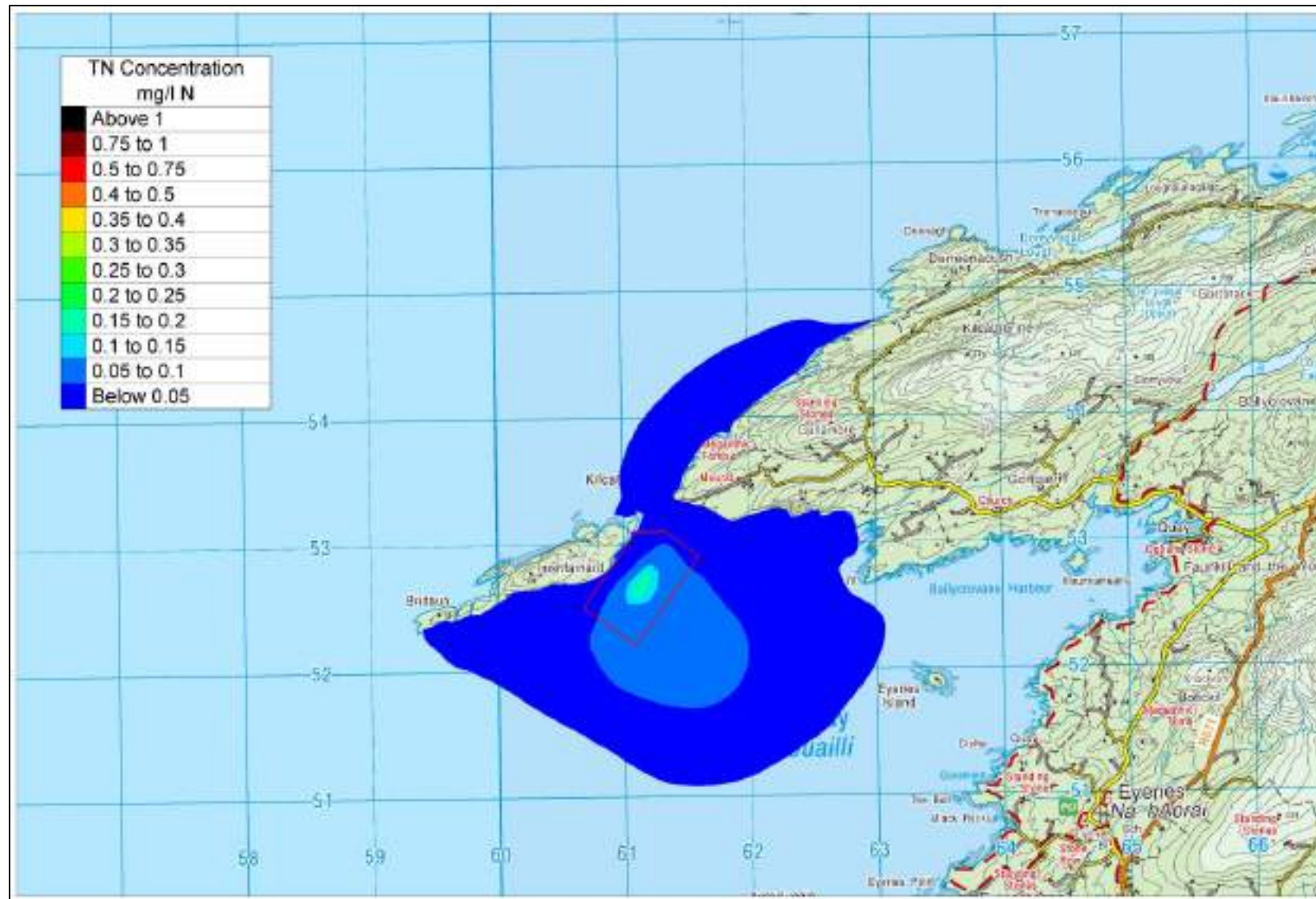
Figure 8-19: Predicted tidal mean total nitrogen concentration envelope (mg/l N) for Inishfarnard Site.
