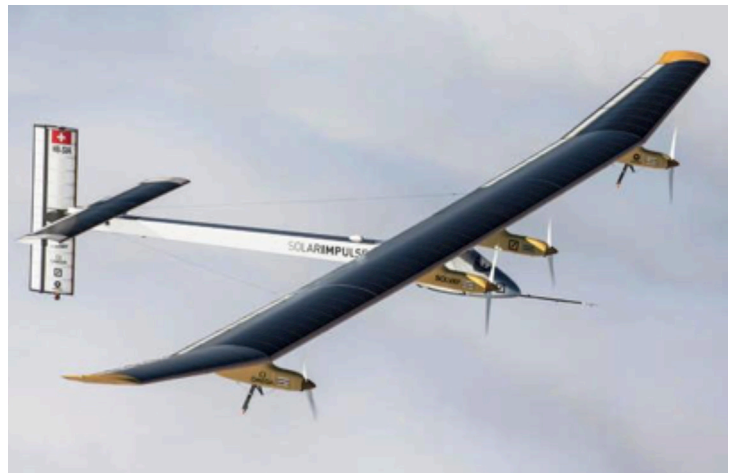
23-3. The wing of the HB-SIA is filled with solar cells used to charge the batteries that power the motors and cockpit electronic systems.
