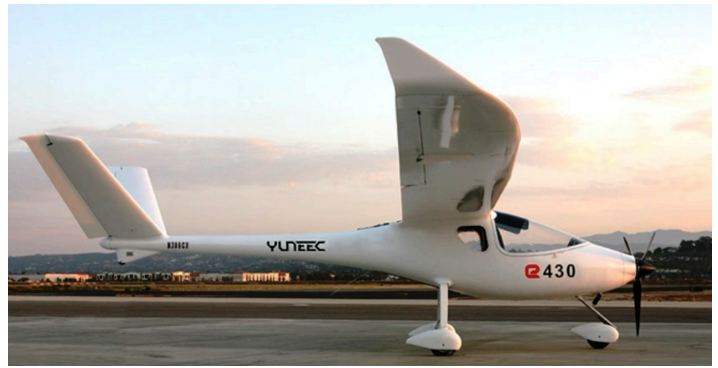
23-6. The E430 uses three lithium polymer battery packs that allow it to fly for two hours in an “optimum cruise” with two people on board.
