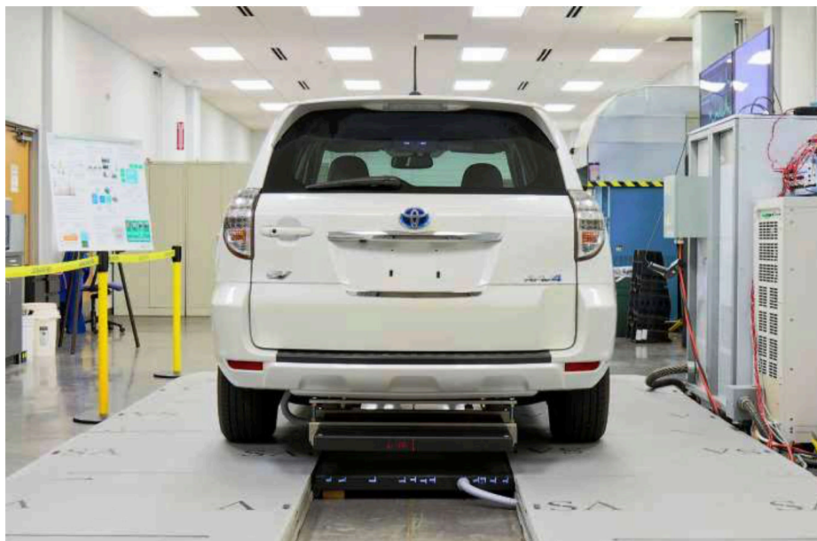
12-3. WPT system installed in an electric Toyota RAV4 equipped with an additional 10kW-hour battery.
