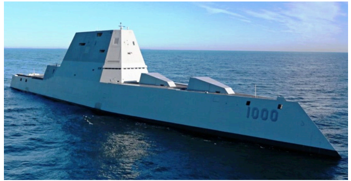
23-12. The U. S. Navy's DDG-1000 has an integrated power system with an all-electric architecture that provides electric power to the total ship (propulsion and ship service) with an integrated plant.
