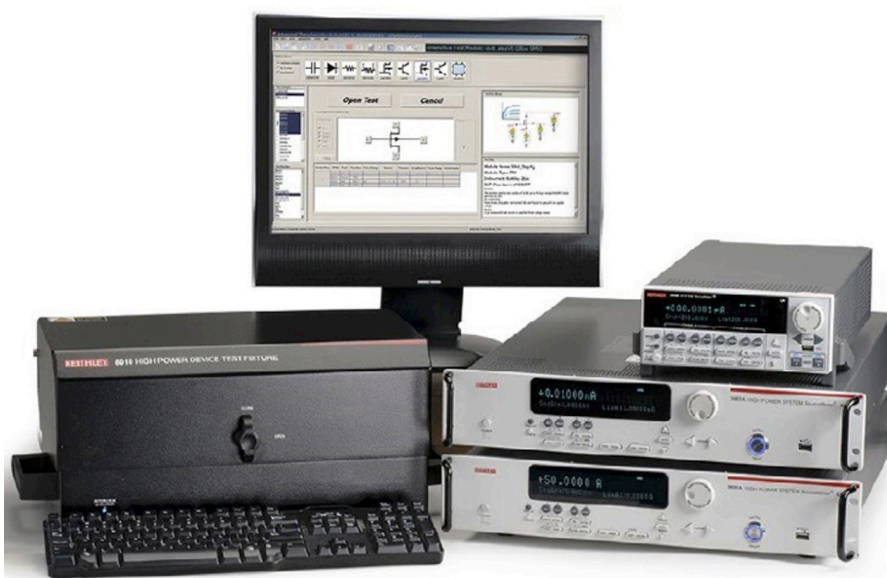
24-12. Tektronix/Keithley's 2600-PCT-xB is intended for characterization of MOSFETS, IGBTs, diodes, and other high-power devices.
