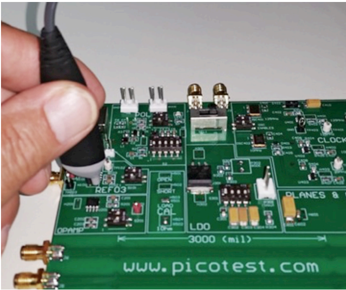
24-4. Picotest's 1-Port probe is used to make an output impedance measurement of a voltage reference.
