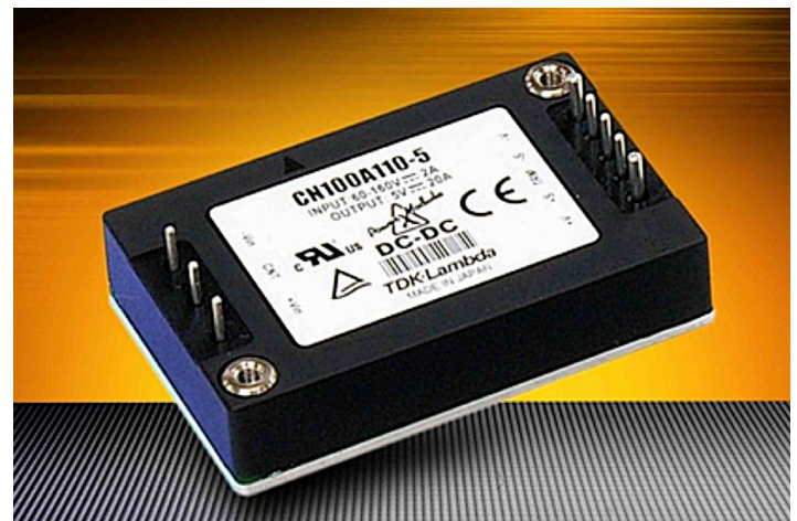
4-1. TDK-Lambda’s CN-A Series of dc-dc converters have a 60V to 160VDC input range with output voltages from 5V to 24VDC (adjustable \pm 10\% ). Output power ratings are 30W, 50W, and 100W. These isolated power modules are in the industry-standard quarter-brick footprint.
