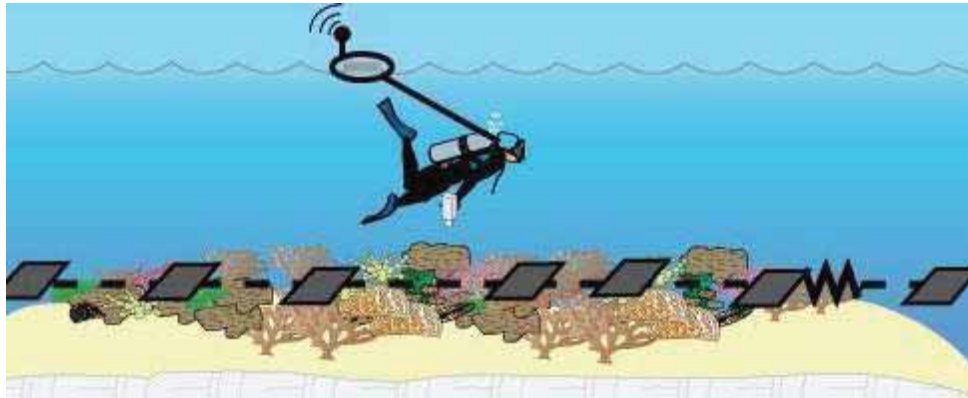
Figure 6: Conceptual diagram of the georeferenced photo transects. Source: (Roelfsema et al. 2014, Roelfsema et al. 2016, Grol et al. 2019)
