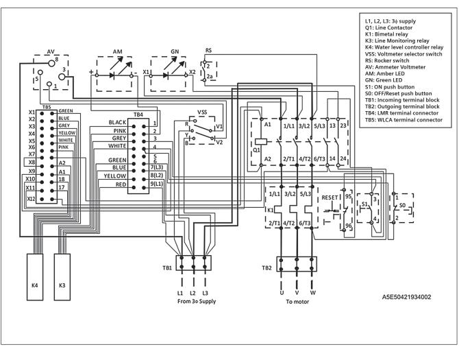
Fig. 4: Wiring Diagram
